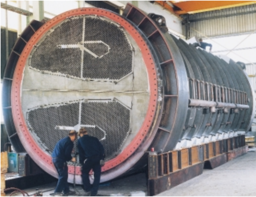
CB/A condenser for Smithfield Energy Facility being manufactured at Evans Deakin's workshop 2
