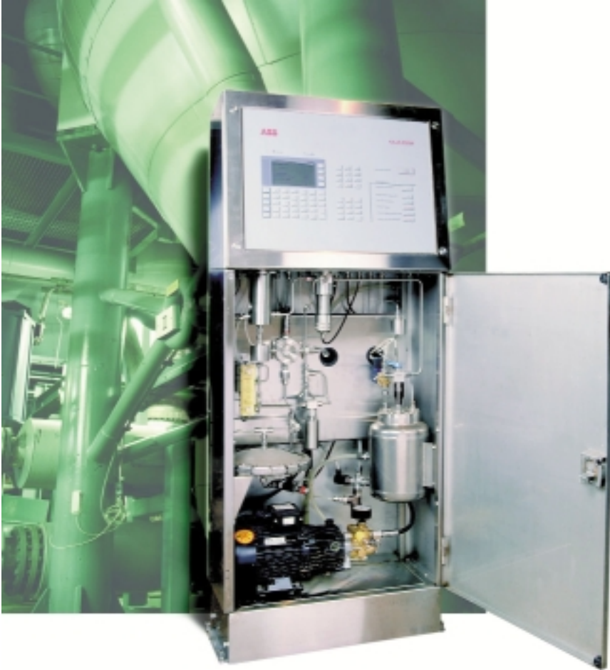
CLA 2000 cooking liquor analyzer. Besides allowing accurate measurement of the liquor concentrations, the CLA 2000 also provides data that assist in the process management.
