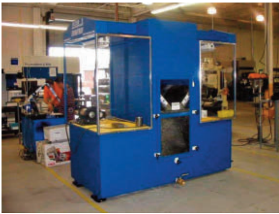
In a wet downdraft table like this, particulates are driven directly into the water below, and clean air is released.
