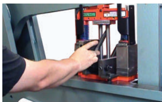
FIGURE 2 A U-bolt is formed with a special bending tool on an ironworker. The bending punch has an open window for the return flange to swing back through during the second bend.
