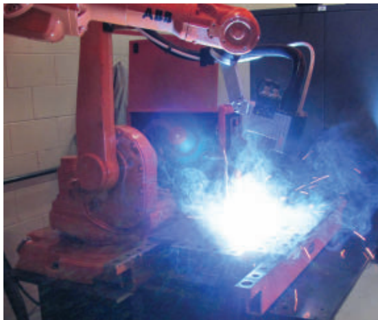
FIGURE 3 A GMAW process with twin wire is a great way to fill large welding gaps often associated with heavy fabrications.
