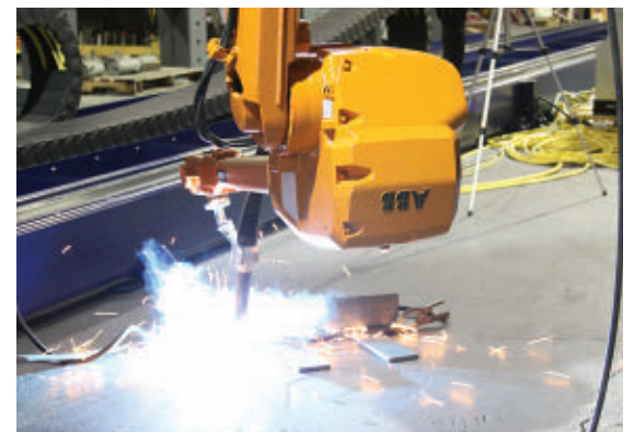
FIGURE 2 Robotic welding torches that rely on tactile sensing typically need only one to three seconds to locate a joint.
