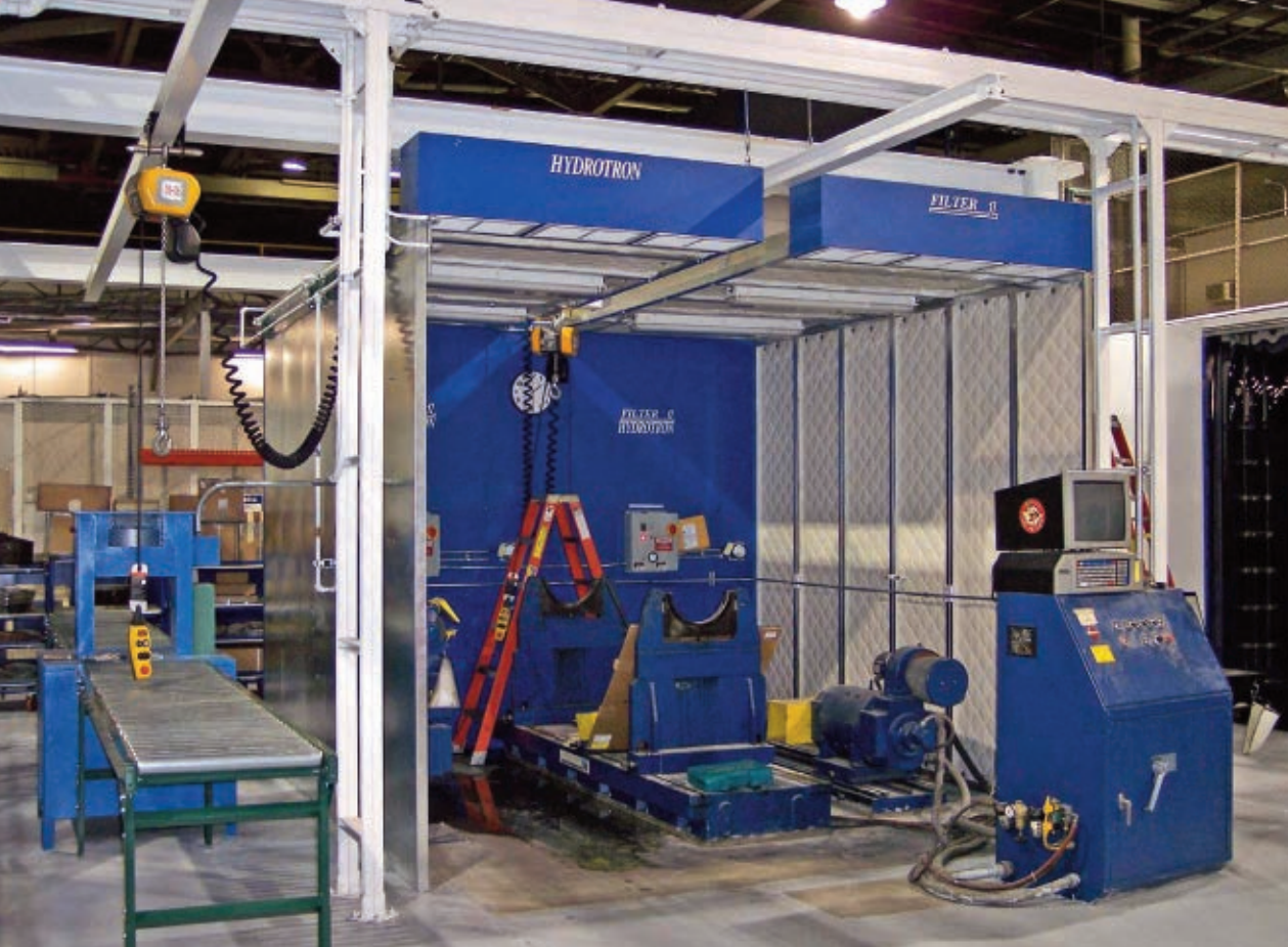
This wet filtration booth works well for applications involving workpieces too large to fit on a typical downdraft table.
