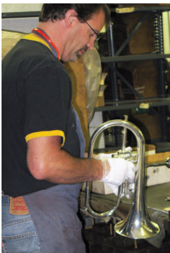
FIGURE 8 An employee performs final lapping on a flugelhorn (the trumpet's larger cousin) to ensure smooth action between the pistons and valve casing.
