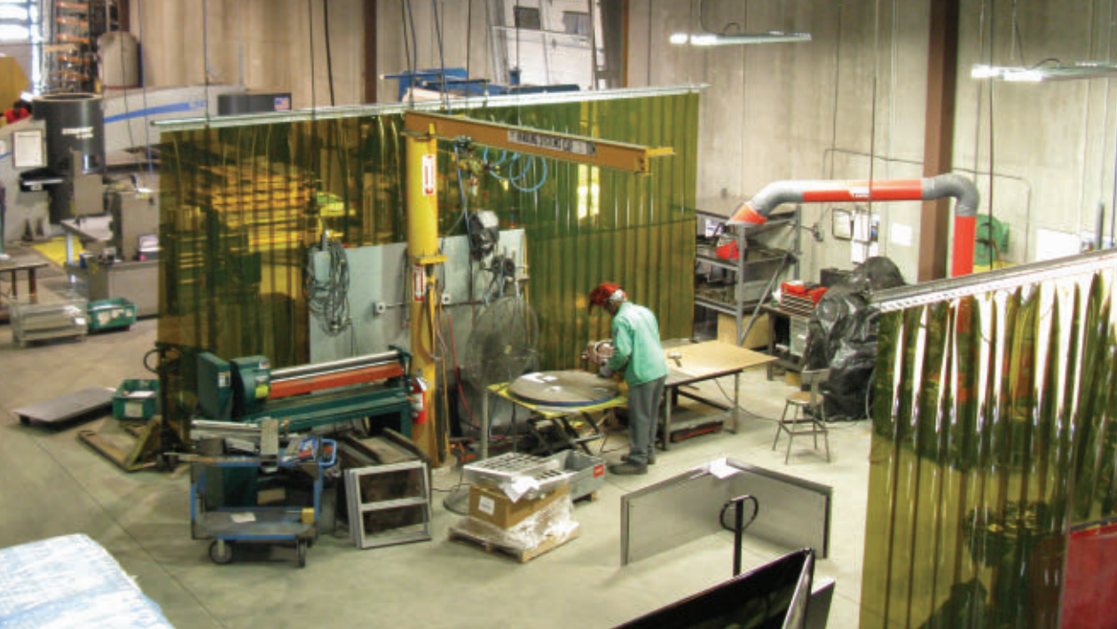
The fabrication cell at Phoenix Products has a punch press, a press brake, and welding stations.
