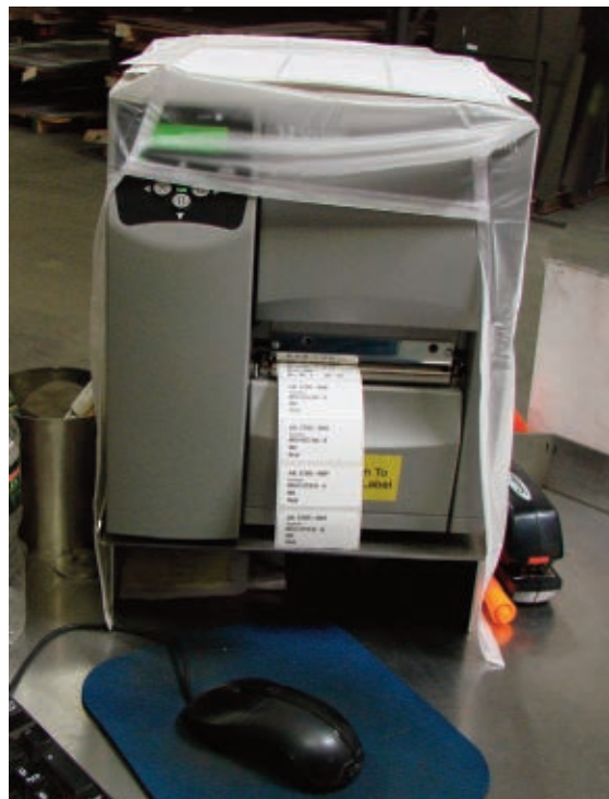
FIGURE 5 A printer adjacent to the laser prints bar code stickers, which are placed on the cut parts that emerge from the laser. The ERP system also replaces estimated material usage from the job quote with the actual amount of metal used for the job, adjusting job cost and inventory data accordingly.
