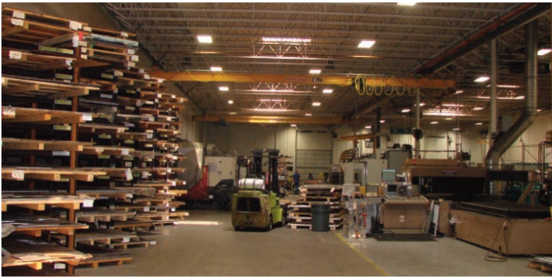
FIGURE 3 Today Anderson carefully organizes its raw stock so that laser machine operators spend more time cutting metal and less time hunting for material.
