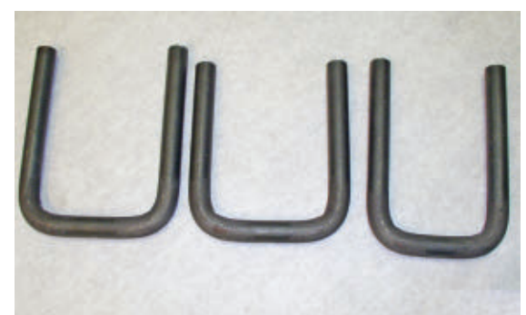
FIGURE 2 A U-bolt is formed with a special bending tool on an ironworker. The bending punch has an open window for the return flange to swing back through during the second bend.
