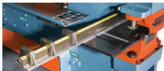
FIGURE 6 This X-Y positioning table helps an operator accurately punch irregularly spaced holes.
