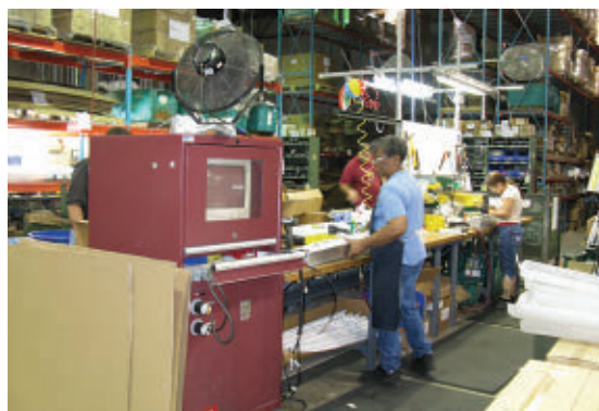
FIGURE 6 In assembly areas all necessary tools are within arm’s reach. More machines were also moved into the area so that workers could complete multiple production steps.
