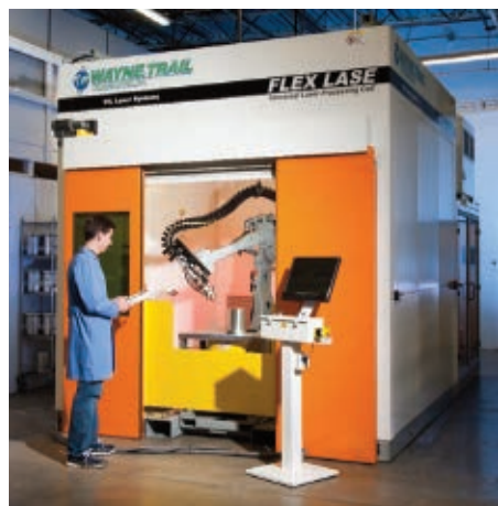
This self-contained, flexible laser processing cell offers a small footprint.
