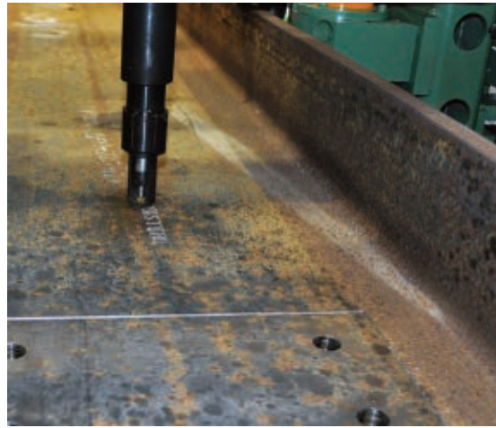
FIGURE 6 A scribe tool places layout markings while the material is on the drilling machine, eliminating the need to mark workpieces manually and expediting fit-up and welding.
