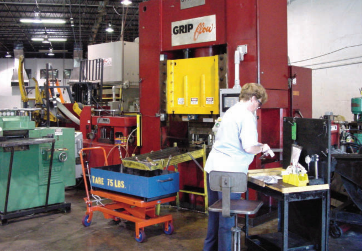
FIGURE 1 The GRIPflow process is sometimes used to form gears and parts that require close flatness tolerances or a square cut edge. Photo courtesy of EBway Corp.
