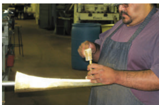
FIGURE 5 A worker hammers a notched bell-stem seam for a trombone.
