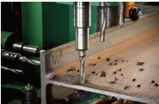
FIGURE 3 Multitool drill lines, such as this nine-spindle system, eliminate downtime and secondary operations for workpieces with multiple hole sizes or operations.
