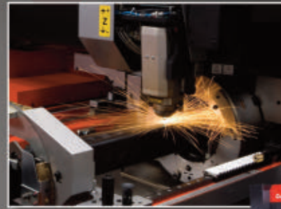
FOM2RI 3015 CO 2 Laser Cutting System The most versatile Rotary Index Laser Cutting System processes round, square, rectangle, C-channel and angle iron
