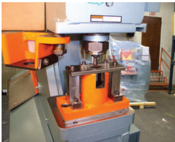
FIGURE 3 This hex punch broaches a predrilled hole to create a hexagon hole in a bolt head. The custom die secures the bolt head as the punch descends.
