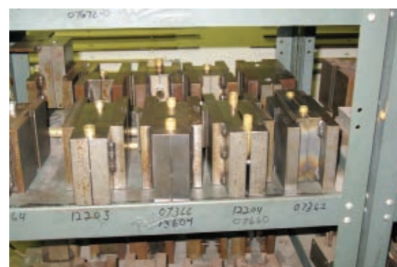
FIGURE 3 These balling-out dies ensure the bent tube's ID is precise.
