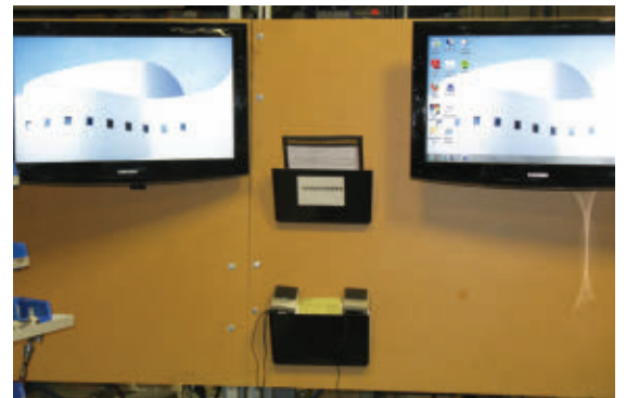
FIGURE 3 Screens in an assembly cell allow workers to pull up complete 3-D models and related information for the job at hand.
