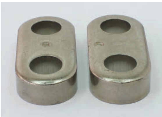
Figure 3 Die roll is typically evident in a part (left) after a punch pierces a hole. In this particular part, the web section is less than 50 percent of the material thickness, which caused additional die roll on the outside contour. EBway created a die that was able to eliminate that die roll in the metal part (right). Photo courtesy of EBway Corp.
