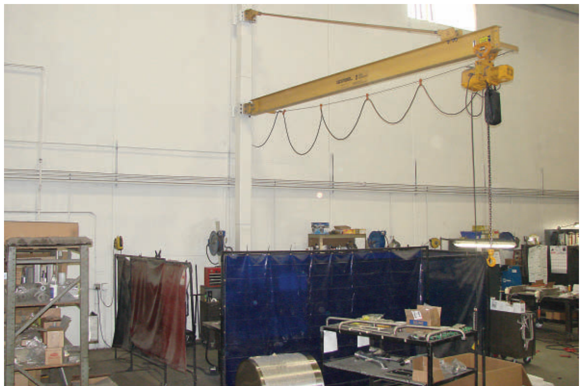
FIGURE 2 Jib cranes adjacent to most welding cells mean welders don't spend time waiting for an overhead crane.
