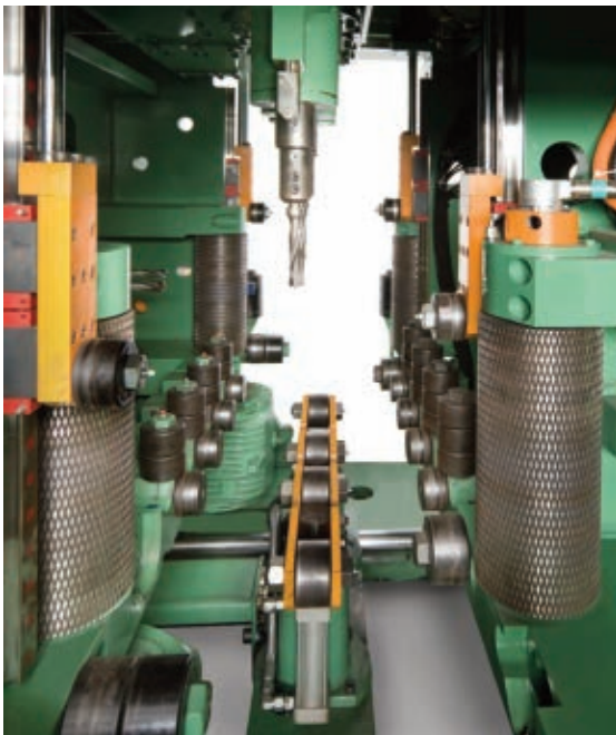
FIGURE 2 For wide profiles, an underside support maintains maximum workpiece stability.
