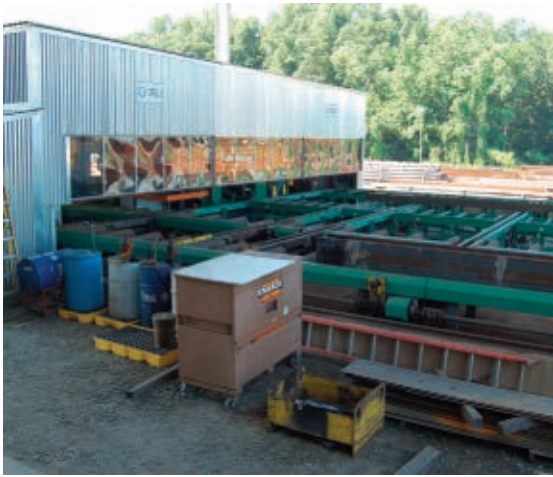
FIGURE 5 A powered conveyor feeds material into two drill and saw lines inside the outbuilding. Not only do such arrangements make for efficient material handling, they also dramatically reduce under-roof area, lowering overhead costs.
