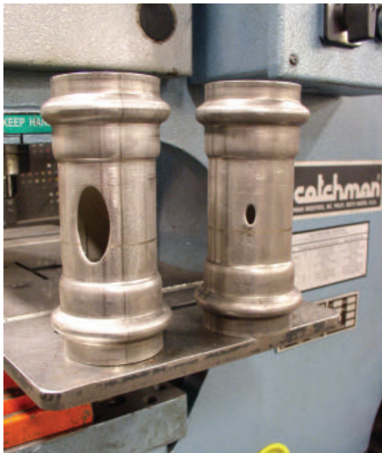
FIGURE 5 This setup punches oval holes into a tube. The mandrel acts as a die and supports the tubular workpiece.
