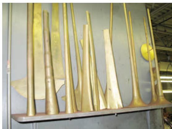
FIGURE 4 The two trombone bell stems on the far left were made from a formed tube. This process does alter the metal thickness, though, so for pro-level horns, bell stems are produced as the remaining work samples illustrate. They start as flat sheet and are bent and hand-hammered into the bell-stem shape.
