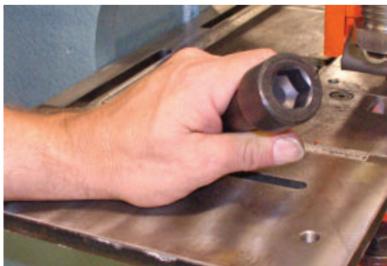
FIGURE 4 The ironworker's custom punch broached a hex shape into this bolt head.
