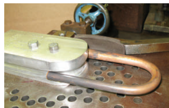
FIGURE 2 Bending the tapered tube of a trumpet bell stem involves pouring a soapy water solution into the ID, freezing it to -65 degrees F, then bending it over the die. The ice doesn't crack during bending because the soap makes it pliable.
