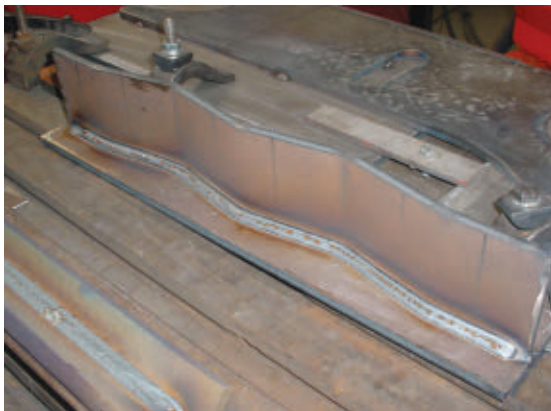
FIGURE 4 This reinforcement plate for an off-road vehicle chassis once took several minutes for a welder to fabricate manually. Now a robotic welding cell can turn out these heavy weldments in a fraction of the time.
