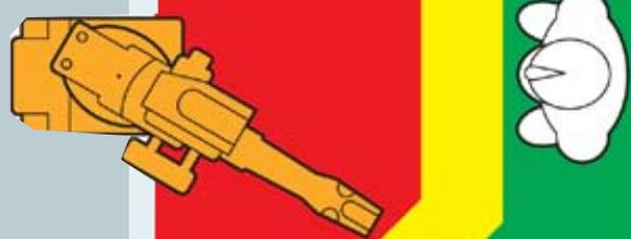
SafeMove confines the robot motion to safe zones, allowing for safe closer interaction between operator and robot.
