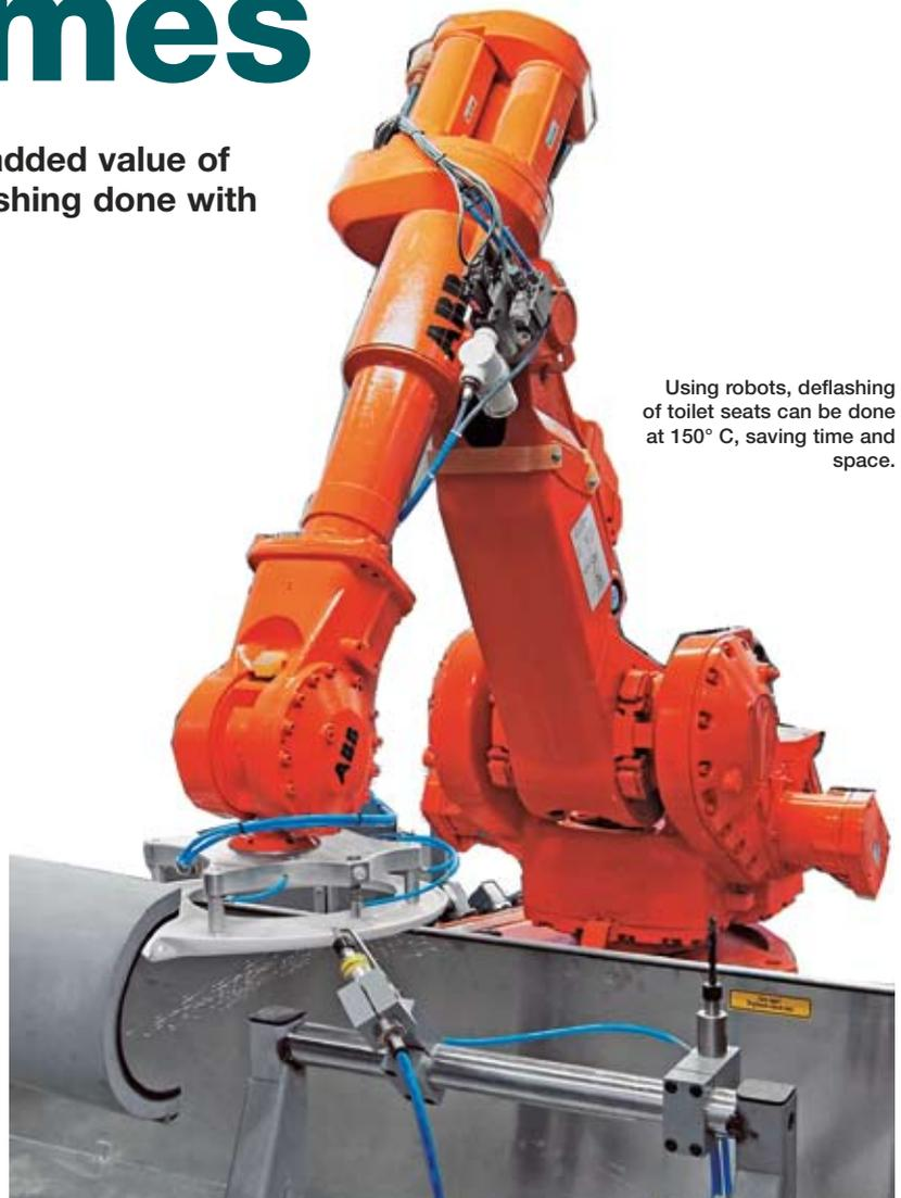
Using robots, deflashing of toilet seats can be done at 150° C, saving time and space.
