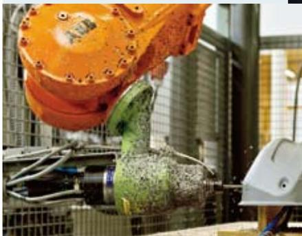
**8** **DISPENSING** Plastic headlamps for India's top automotive manufacturers are glued together by robots at Lumax.
