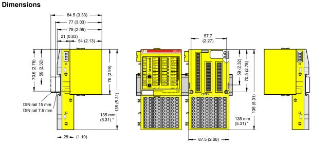
Fig. 61: Dimensions of TU582-S Safety I/O Terminal Unit
