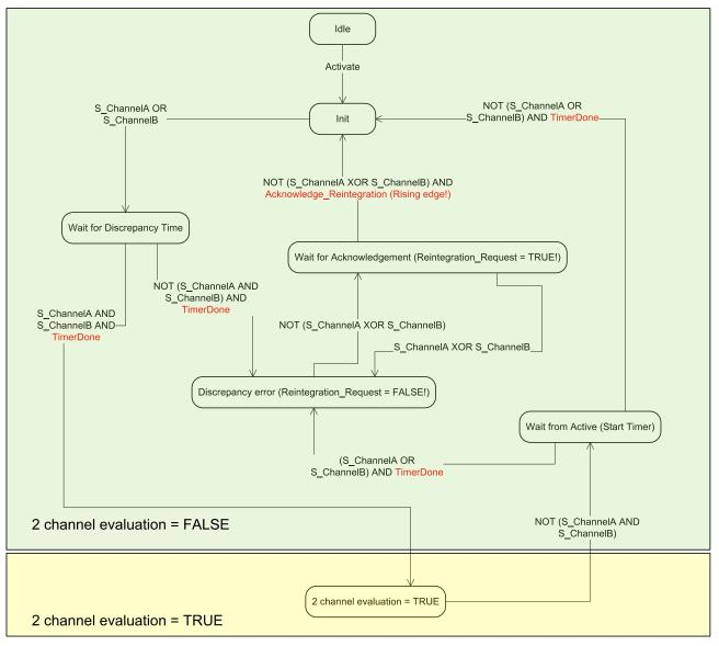
Fig. 17: 2 channel equivalent mode implemented in DI581-S
