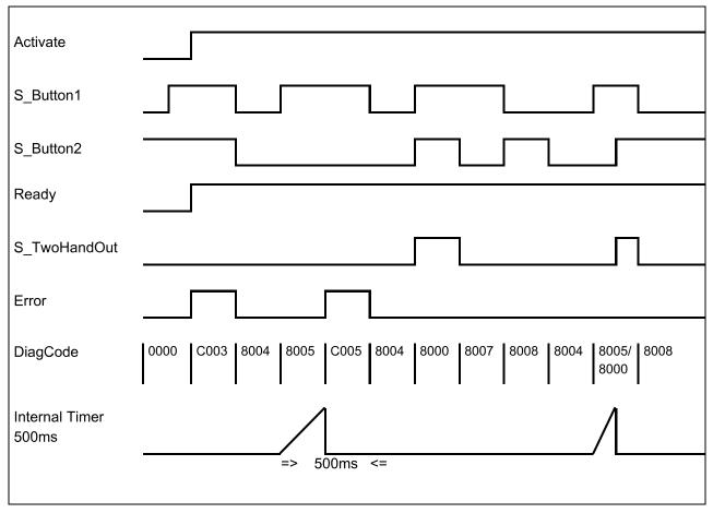
Fig. 111: Timing diagram for SF\_TwoHandControlTypeIII
