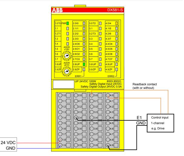
Fig. 46: Circuit example DX581-S, Transistor input (1-channel)
