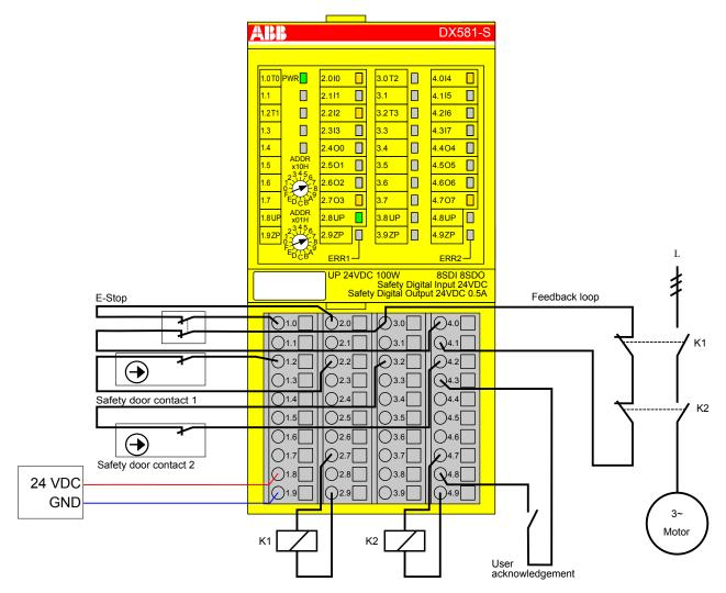
Fig. 48: Application example with DX581-S
