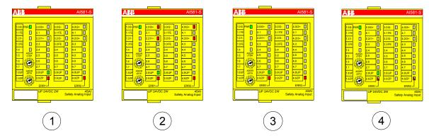
Fig. 15: LED states of Safety I/O modules during start-up (example with AI581-S module)
