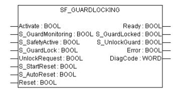
This FB controls an entrance to a hazardous area via an interlocking guard with guard locking ("four state interlocking").
