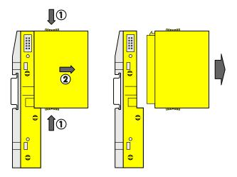
Fig. 20: Disassembly instructions
