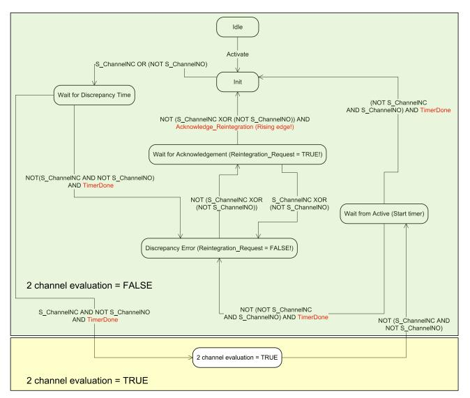
Fig. 18: 2 channel antivalent mode implemented in DI581-S
