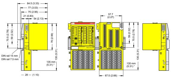
Fig. 52: Dimensions of AI581-S Safety I/O module
