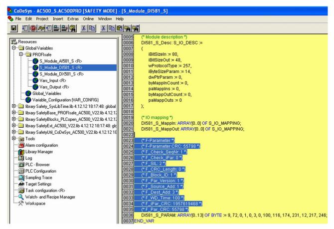
Fig. 87: F-Parameter values in CoDeSys Safety V2.3
