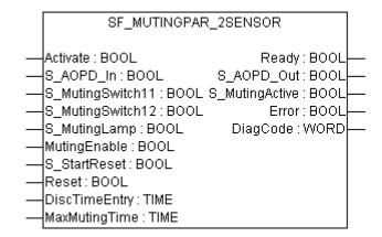
Muting is the intended suppression of the safety function. In this FB, parallel muting with two muting sensors is specified.
