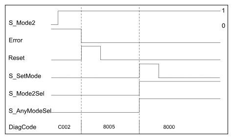
Fig. 102: Timing diagram for SF\_ModeSelector, reset of error condition
