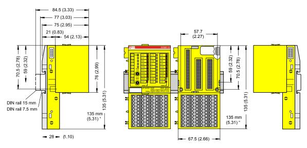
Fig. 41: Dimensions of DX581-S Safety I/O module
