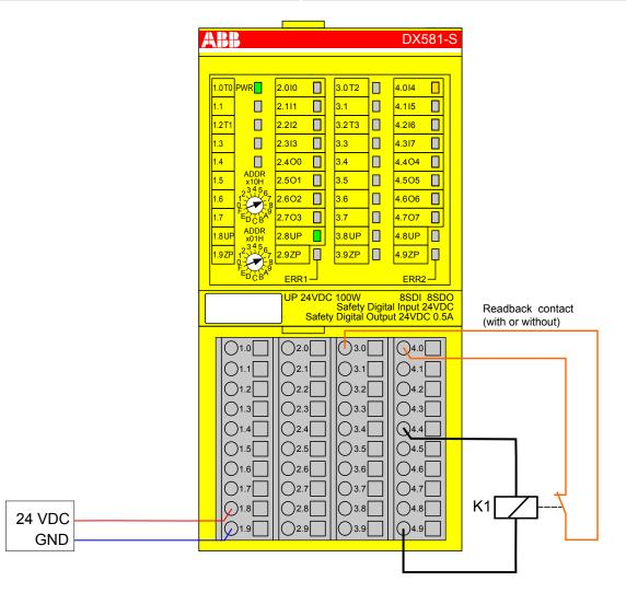
Fig. 44: Circuit example DX581-S, Relay
