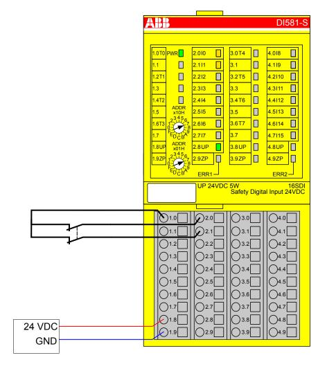
Fig. 30: Circuit example DI581-S, 2-channel sensor (equivalent) with test pulses
