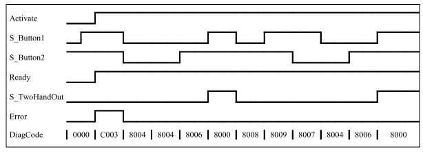
Fig. 110: Timing diagram for SF\_TwoHandControlTypeII
