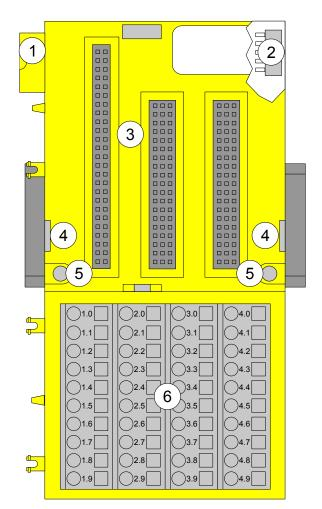
Fig. 59: Safety I/O Terminal Unit TU582-S (spring-type) for Safety I/O expansion modules
