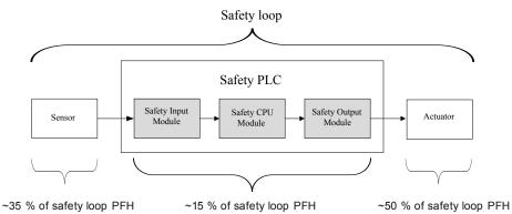
Fig. 3: Typical safety loop with AC500-S Safety PLC
