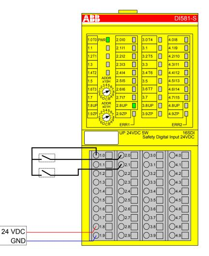
Fig. 33: Circuit example DI581-S, 2 separate sensors with test pulses
