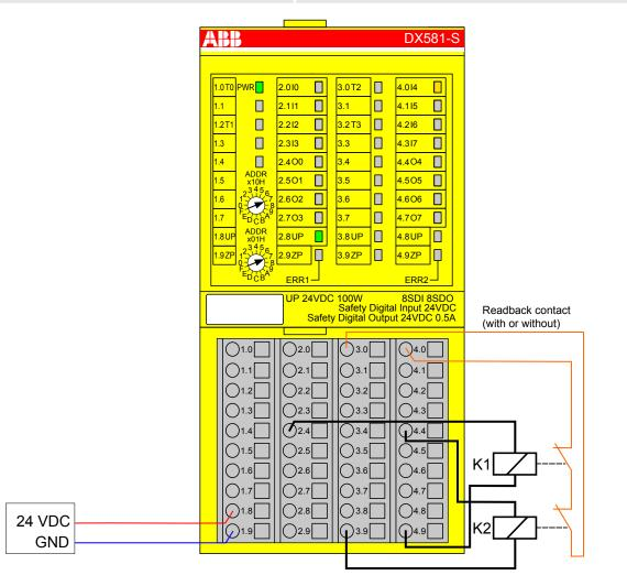
Fig. 45: Circuit example DX581-S, Relay (2-channel redundant)
