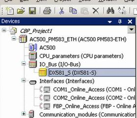
2. Go to the iParameter setting tab (DX581-S, DI581-S or AI581-S respectively) for the given module and set appropriate iParameter values (e.g., *"Test Pulse"*, *"Input Delay"*, etc.).
