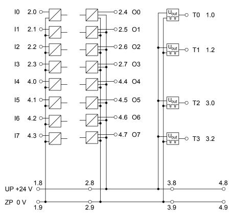
Fig. 42: Example of electrical connections with DX581-S
