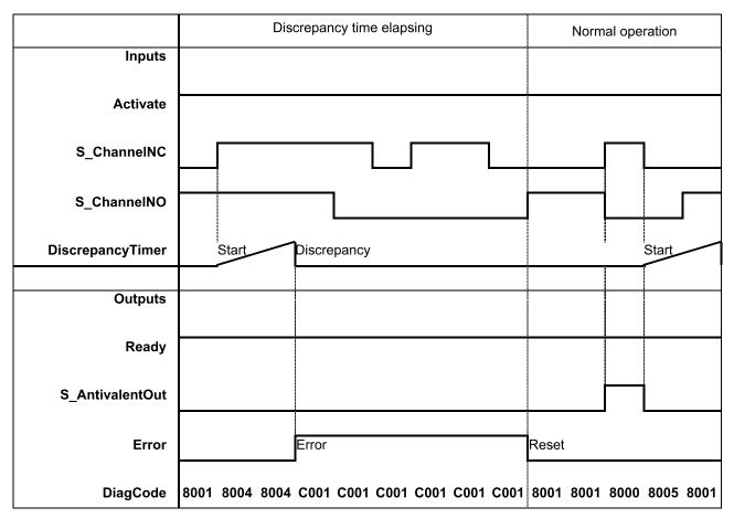
Fig. 99: Typical Timing Diagram for SF\_Antivalent
