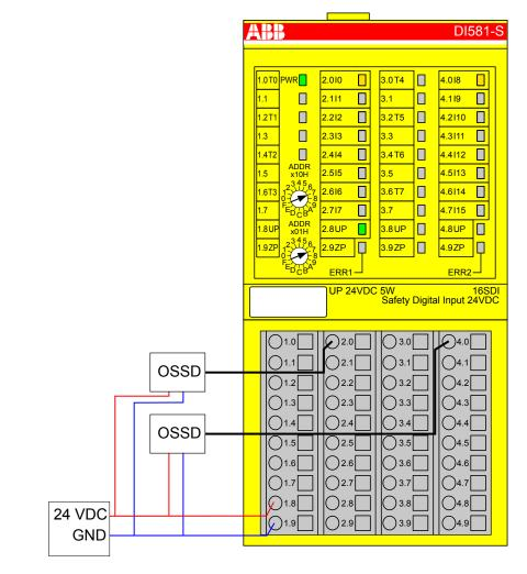
Fig. 32: Circuit example DI581-S, 2 x OSSD output (with internal tests), external sensor power supply
