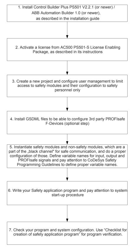
Fig. 63: AC500-S system configuration and programming workflow
