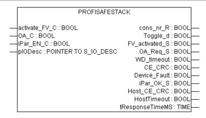
This function block represents PROFIsafe F-Device instance in the PROFIsafe F-Host to control and monitor the status of the given F-Device [3].
