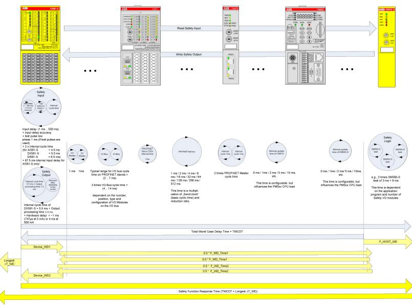
Fig. 127: SFRT in AC500-S system with PROFINET components
