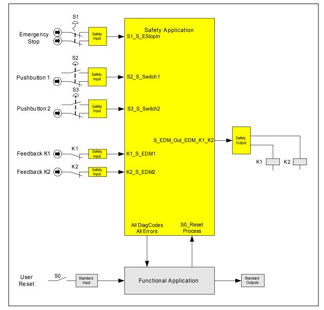
Fig. 139: Graphical overview of the example TwoHand Control with EDM
