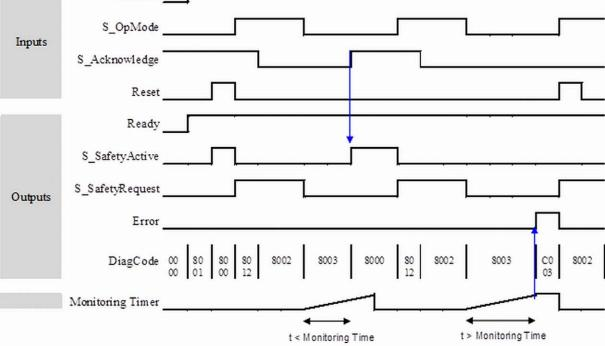
Fig. 121: Timing diagram for SF\_SafetyRequest
