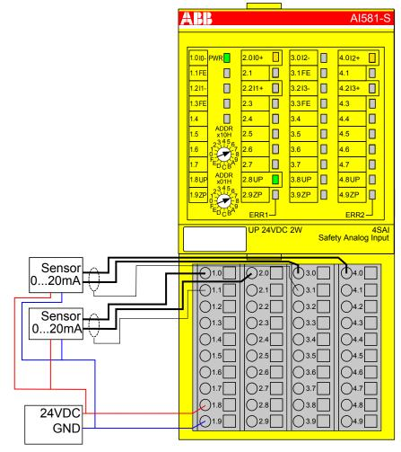
Fig. 56: Circuit example AI581-S, 2 analog sensors (0 ... 20 mA)
