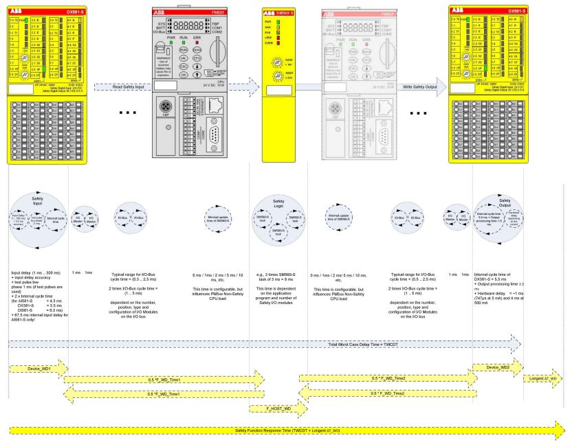
Fig. 126: SFRT in AC500-S system without PROFINET components
