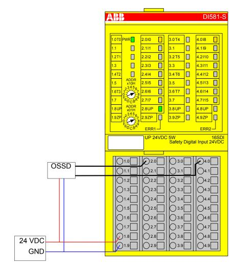
Fig. 28: Circuit example DI581-S, 2-channel OSSD output (with internal tests), external sensor power supply
