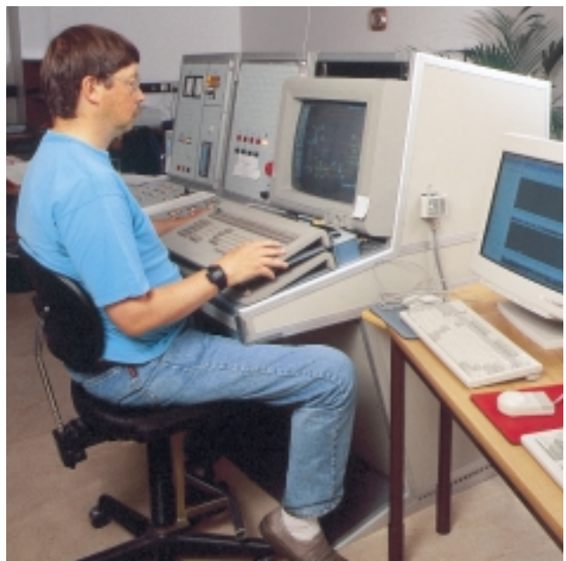
New control room at the FRIGG test facility. Control is by means of ABB Master. The rod temperatures are monitored on the screen on the right.
