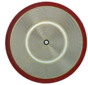
1b Top view of a 91 mm IGCT wafer
