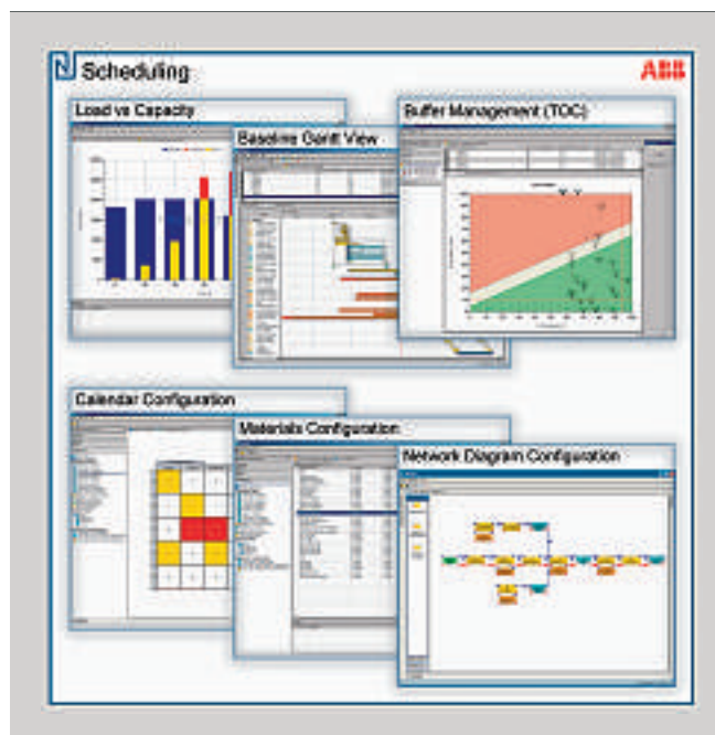
2 Scheduling system providing full support for TOC and Finite Capacity approach
