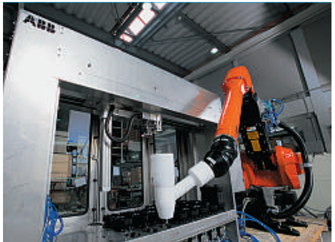
2 A paint robot changing its cartridge in the manipulator. The empty cartridge is automatically refilled
