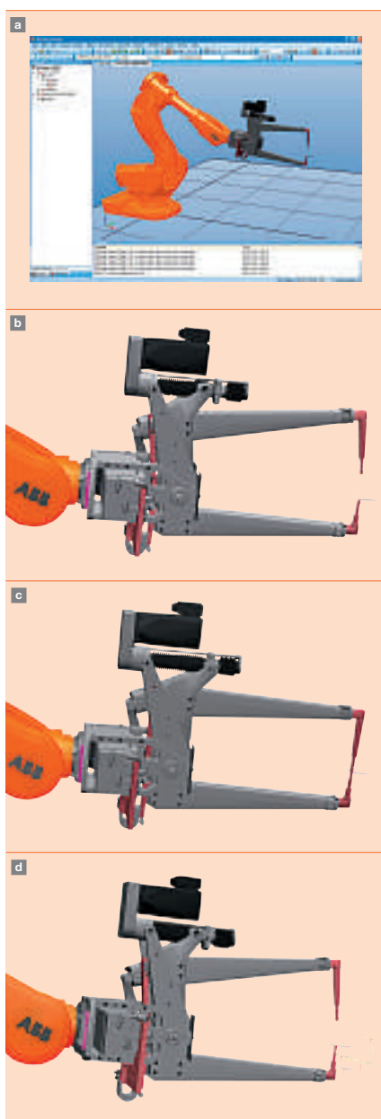
2 Views of a typical spotwelding cycle, created with ABB's RobotStudio software
