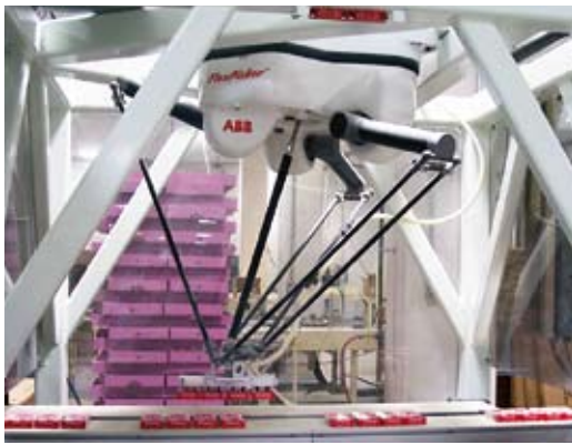
The IRB 340 picks up four packs of Sweethearts at a time, orienting the boxes depending on the wrapping used.
