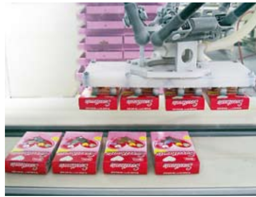
The IRB 340 picks up four packs of Sweethearts at a time, orienting the boxes depending on the wrapping used.
