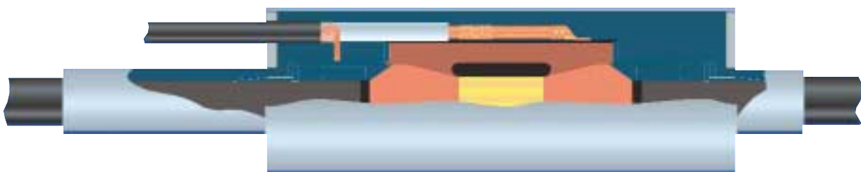
4 This prefabricated EHV cable joint, developed by ABB, contains neither gaseous nor liquid materials and is maintenance-free.
