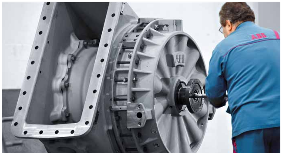
3 PTL power turbines are built in ABB’s modern factory in Switzerland
