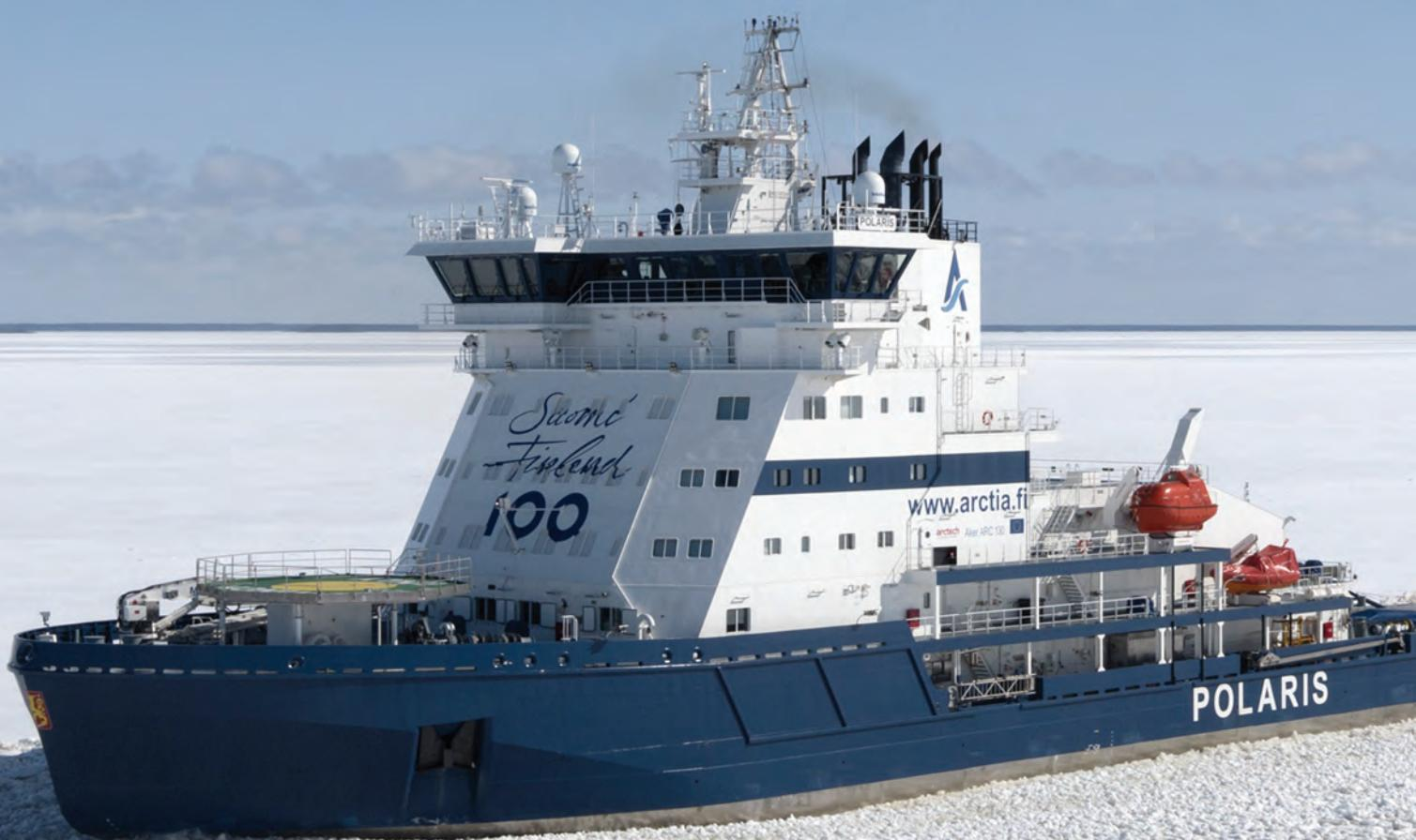
seldom comes easy. “LNG adds both costs and complicating issues to design,” says Mika. “Like how to accommodate larger tanks on the ship.” LNG requires more volume for the same amount of energy as fuel oils, and the pressurised tanks required to contain it take up more space. “The rule of thumb is four times the volume of fuel oils.”
