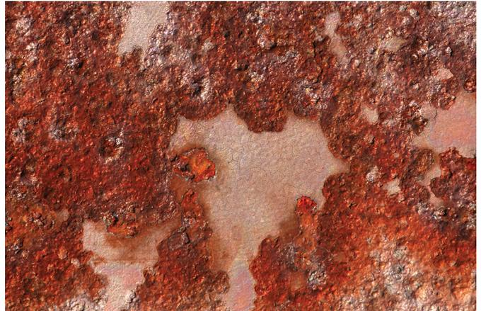
In its dissolved form, oxygen is highly corrosive to most metals, especially the mild steel used for boiler tubes.
