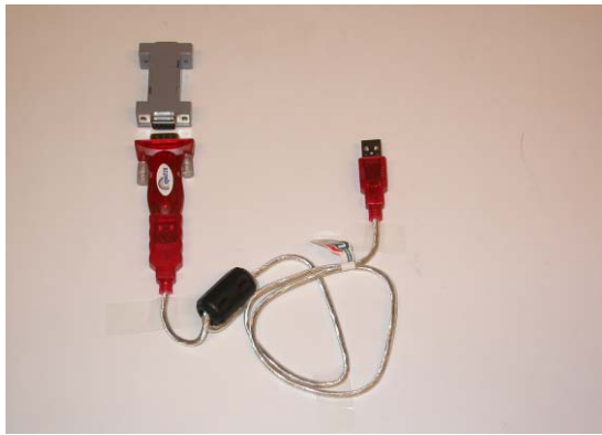
USB/485 Half Duplex converter cable - male D-Sub 9-pin connector D-Sub 9-pin interfacing adapter.
