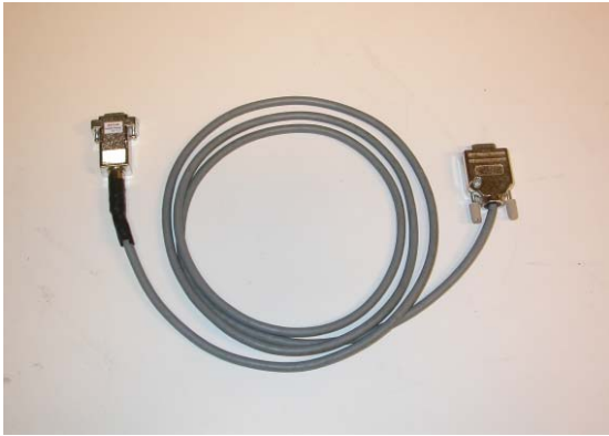
RS232/485 Half Duplex converter cable - male D-Sub 9-pin connector.
