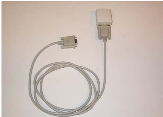
ABB optic cable RS232/IrDA converter and D-Sub 9-pin extension.
