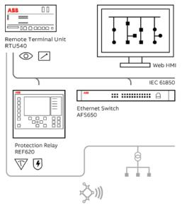
functionality provides a perfect overview of the status of the distribution network. Adding protection applications ensures power is only interrupted when absolutely necessary, to provide the highest reliability and quality of service for customers.
