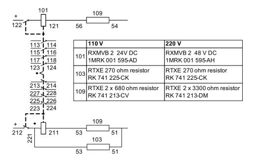
Handling of capacitive discharge currents intorelay by using parallel resistor (103)
