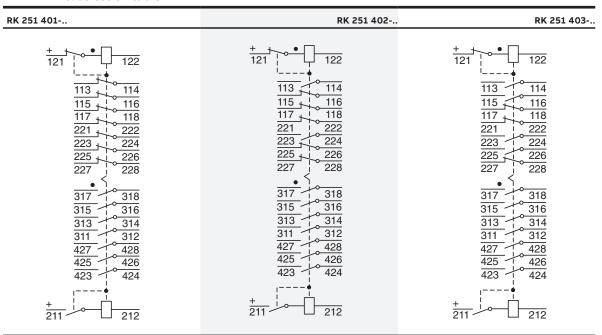
When the winding terminal marked with a dot is positive the contact moves to the position marked with a dot.
