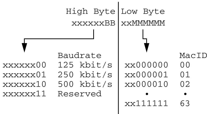
For example, a baudrate of 250 kbit/s and MacID 63 are entered as follows:
