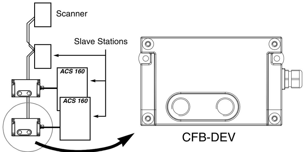
Figure 2-2 The construction of the DeviceNet link and the CFB-DEV DeviceNet Adapter Module.
