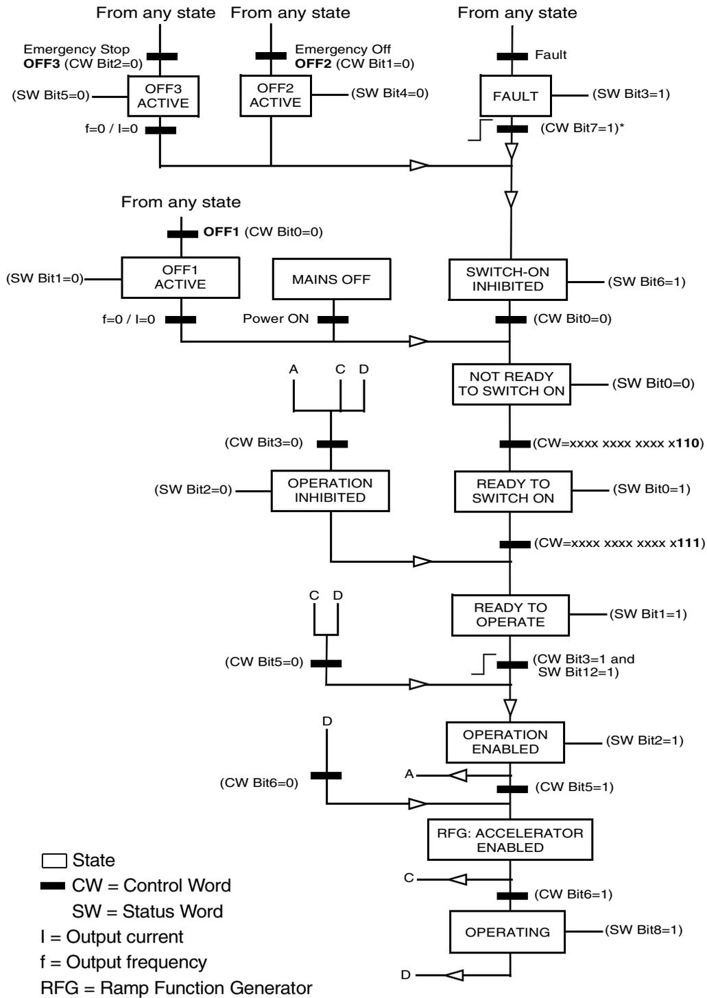
\*This state transition occurs also if the fault is reset from any other source (e.g. digital input).
