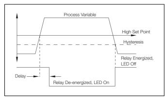
Fig. 5.3 High Failsafe Alarm with Hysteresis and Delay
