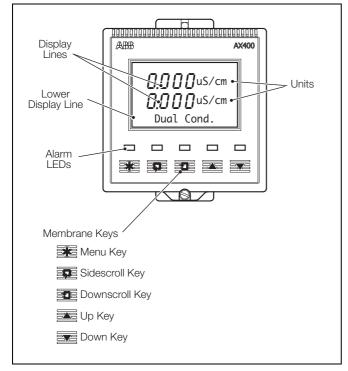
Fig. 2.1 Location of Controls and Displays
