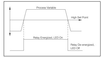
Fig. 5.4 High Non-Failsafe Alarm without Delay and Hysteresis
