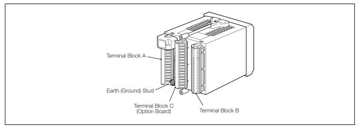
Fig. 6.10 Access to Terminals, Panel-mount Analyzers
