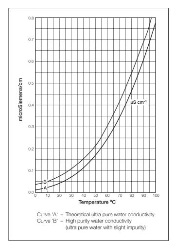
Fig. A.1 Ultra-pure Water Temperature Compensation
