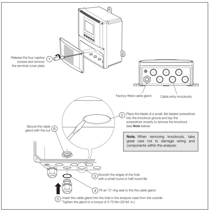
Fig. 6.7 Cable Entry Knockouts, Wall-/Pipe-mount Analyzer
