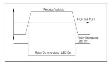
Fig. 5.1 High Failsafe Alarm without Hysteresis and Delay
