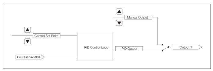
Fig. B.1 Single PID Controller
