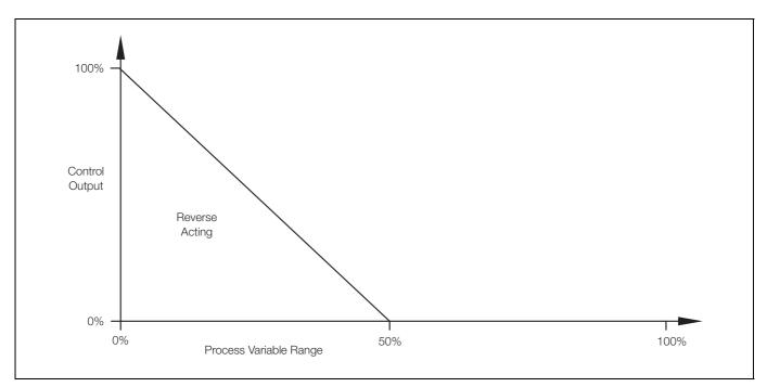
Fig. B.2 Reverse Acting Single PID Control
