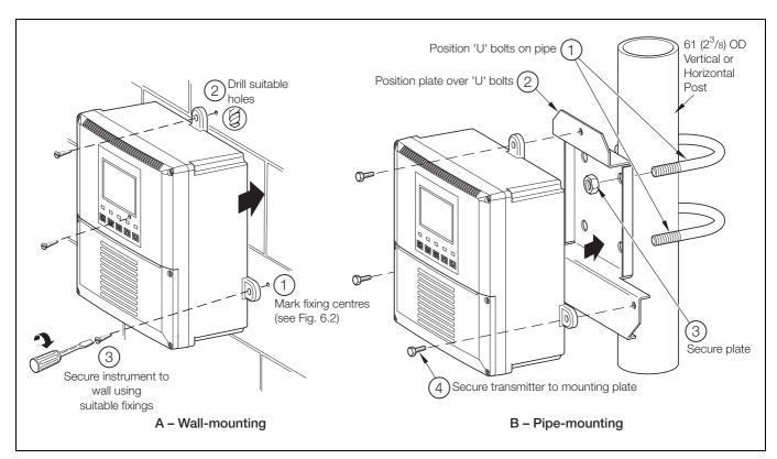
Fig. 6.3 Wall-/Pipe-mounting
