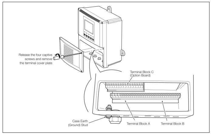
Fig. 6.8 Access to Terminals, Wall-/Pipe-mount Analyzer
