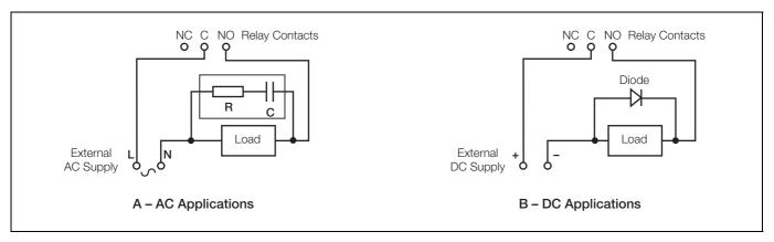
Fig. 6.6 Relay Contact Protection
