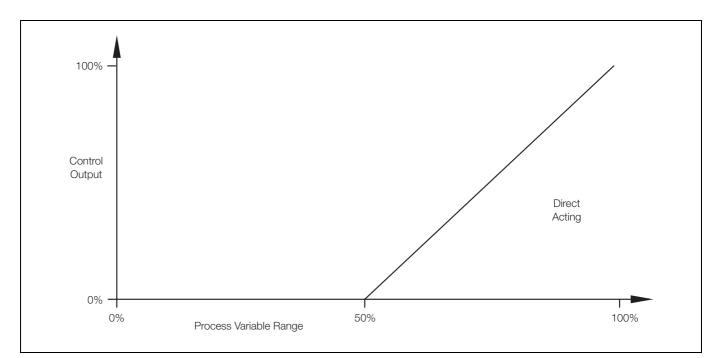
Fig. B.3 Direct Acting Single PID Control
