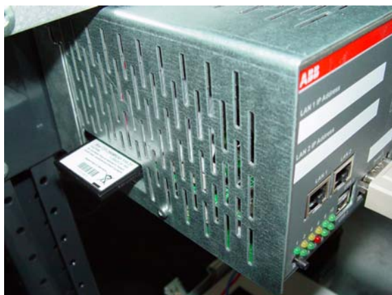
Figure 13 CF card insertion
