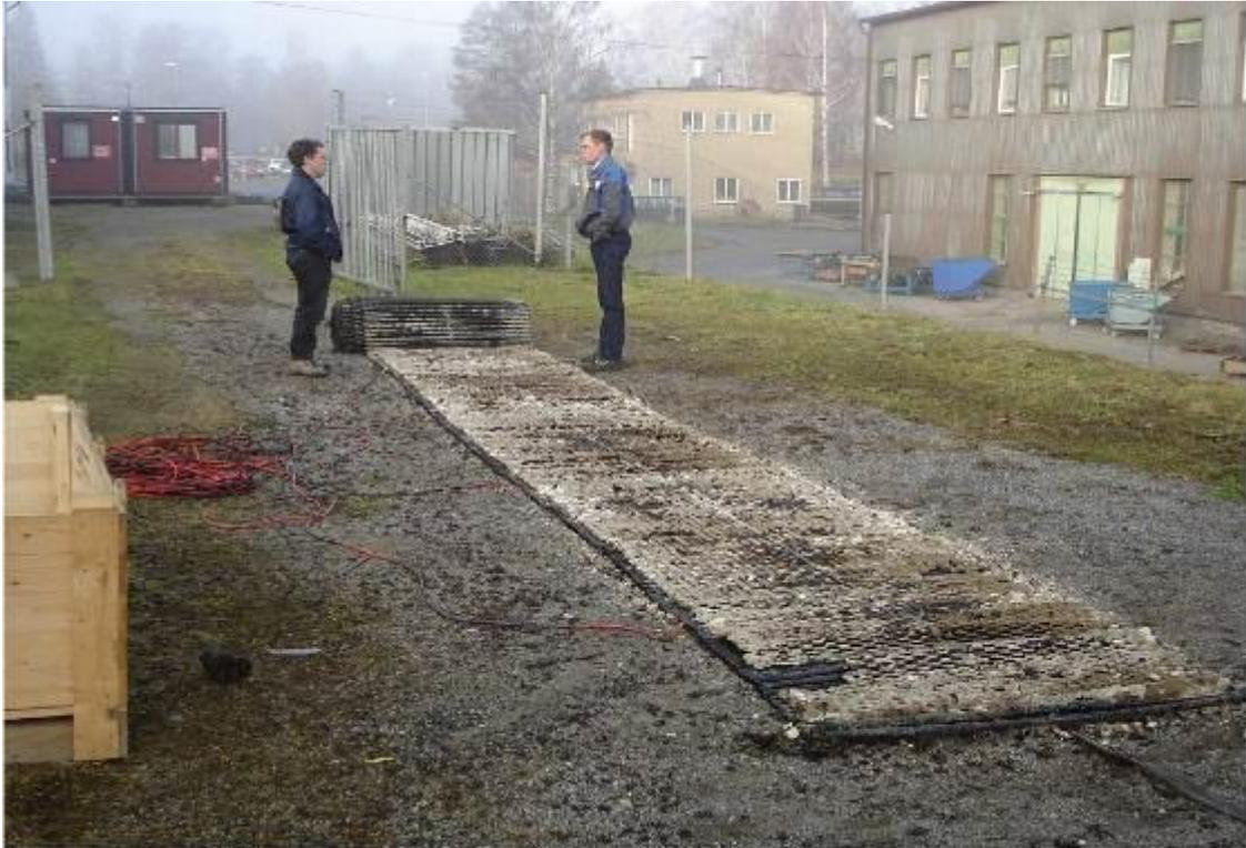
Figure 6 Test electrode titanium net after 20 years operation in cathode mode
