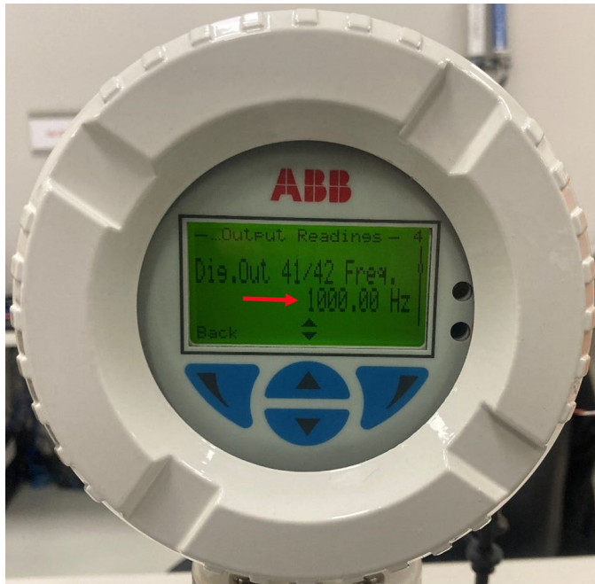
Figure 7-2: ABB CoriolisMaster DO 41/42 frequency output
