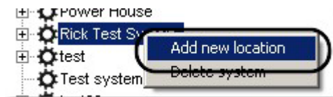
Figure 19 - Adding a location to the system configuration
