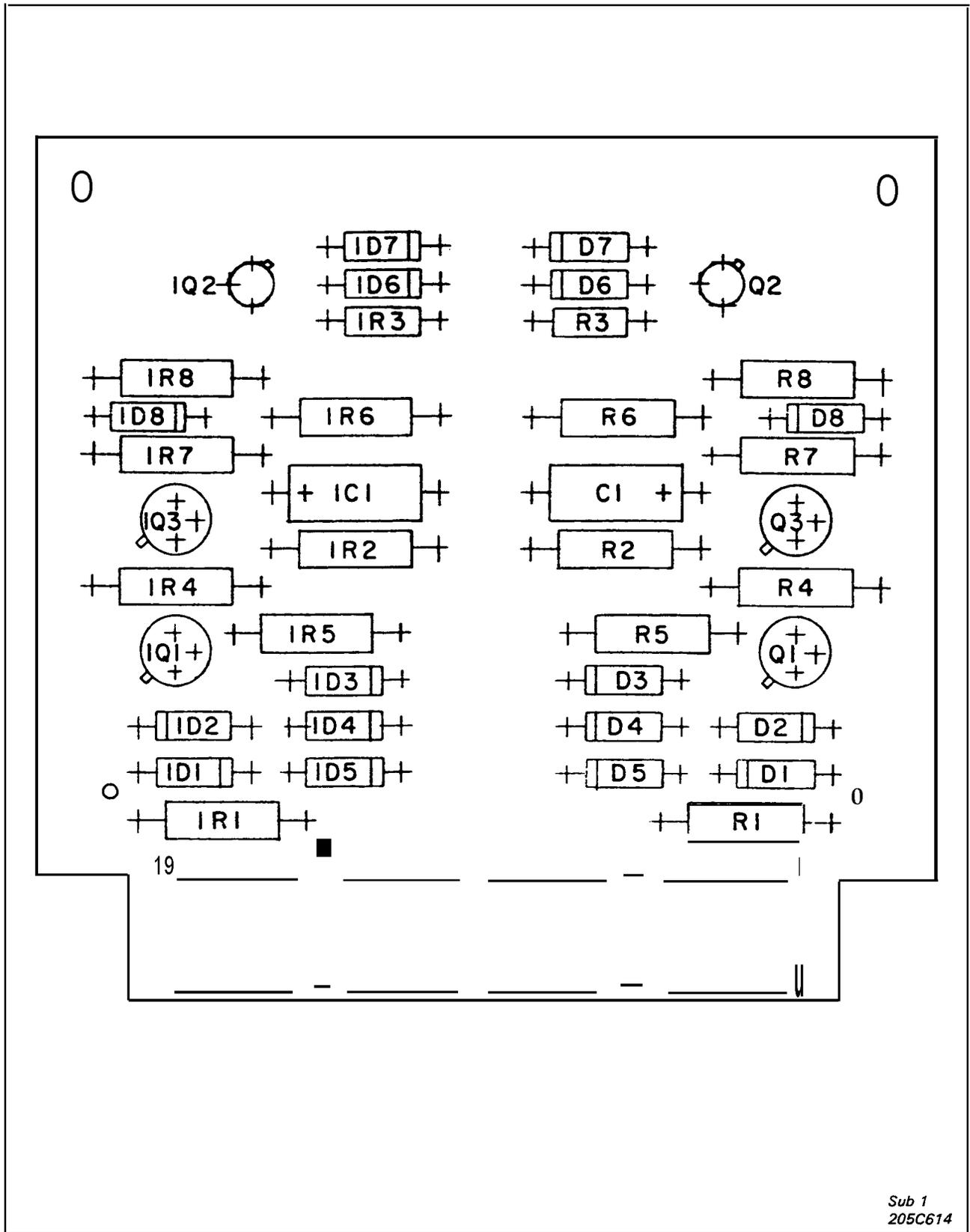
Fig. 11. Component Location (Timer Board).
