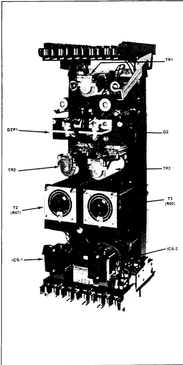
Fig. 1. SLB Relay (2 Timer) Chassis (Front View).
