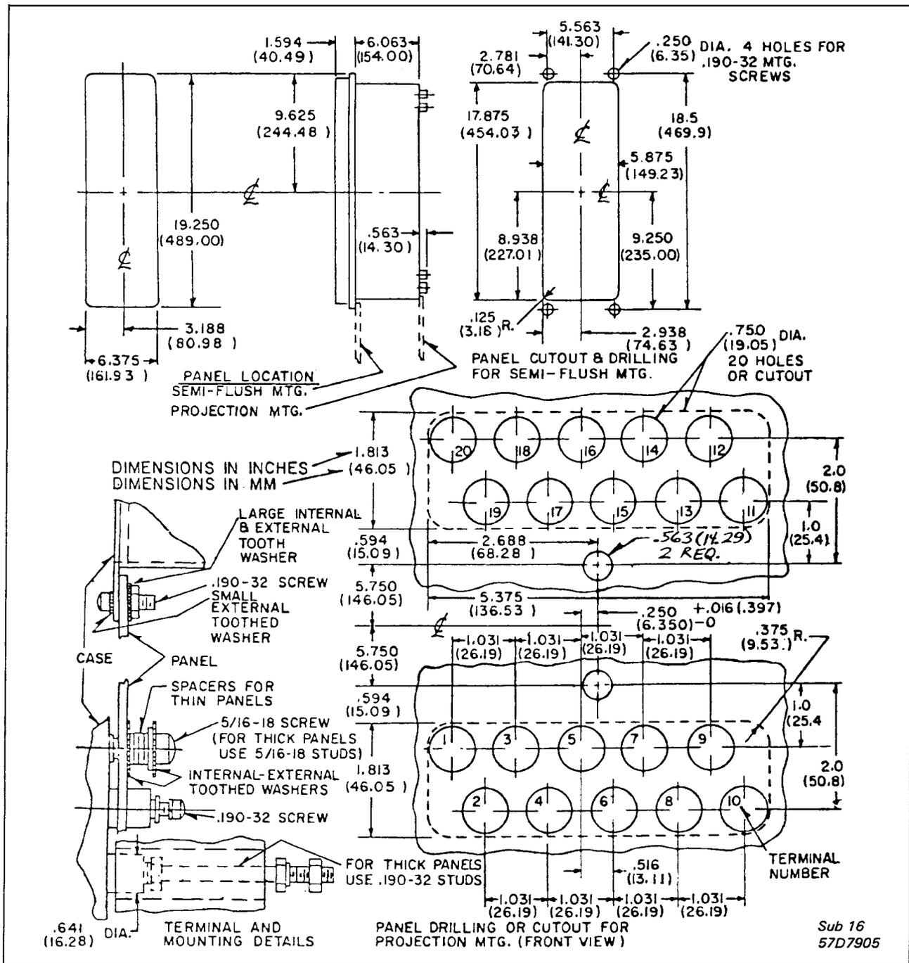
★ Fig. 15. Outline and Drilling Plan for Type SLB Relay in Type FT-42 Case.
