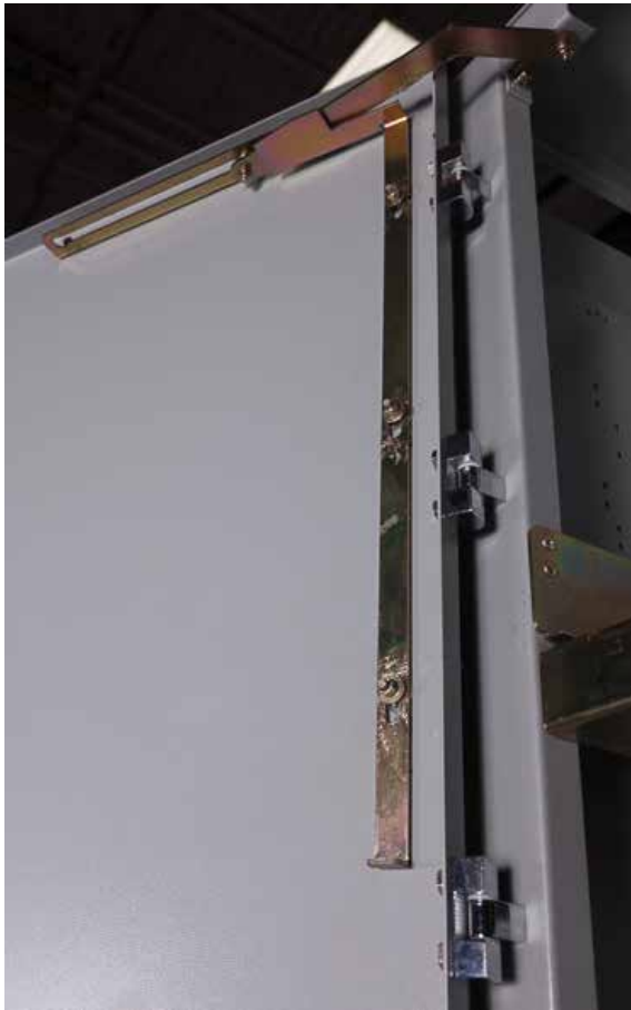
Figure 6-6: Door Stop and Hinges
