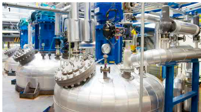
1 Pressurized batch reactors | 2 Powder dosing hopper with bag emptying | 3 Drum filling line | 4 Pig launching station, heat traced and insulated
