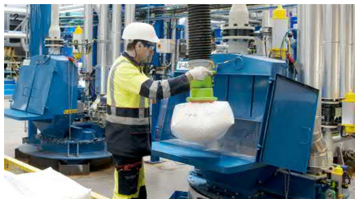
1 Pressurized batch reactors | 2 Powder dosing hopper with bag emptying | 3 Drum filling line | 4 Pig launching station, heat traced and insulated
