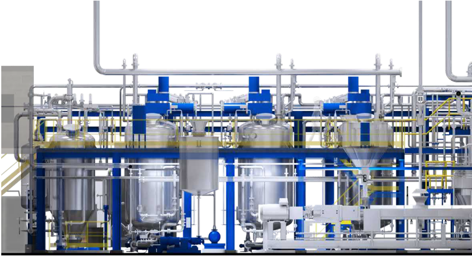
Batch and continuous grease manufacturing plant with common storage tanks and filling lines
