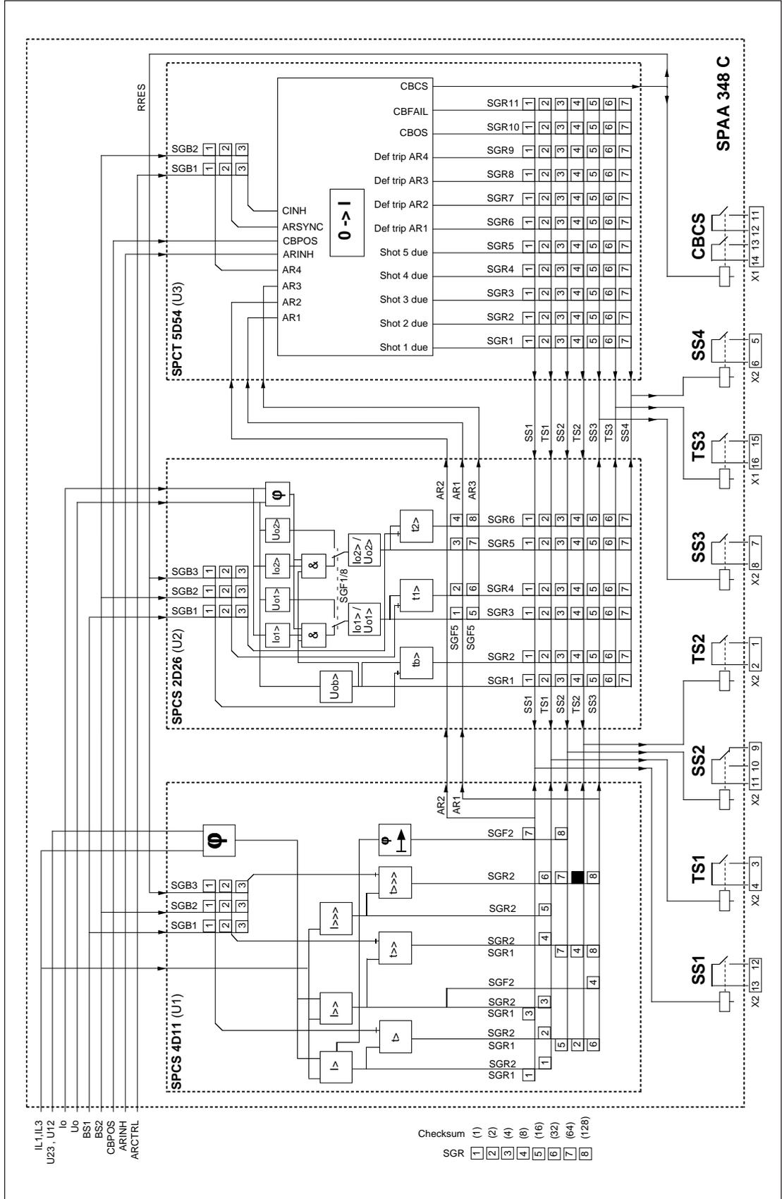
Fig. 4. Internal signals of feeder protection relay SPAA 348 C.
