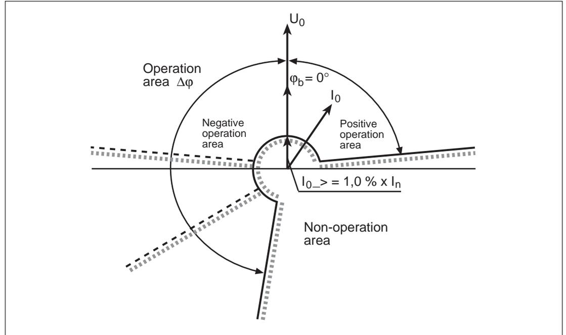
Fig.1. Example of three operation areas:  $\Delta\phi$ ,  $-80^\circ \dots 0^\circ \dots +80^\circ$ ,  $-120^\circ \dots 0^\circ \dots +80^\circ$  and  $-170^\circ \dots 0^\circ \dots +80^\circ$ , when the basic angle is  $\phi_b = 0^\circ$ .
