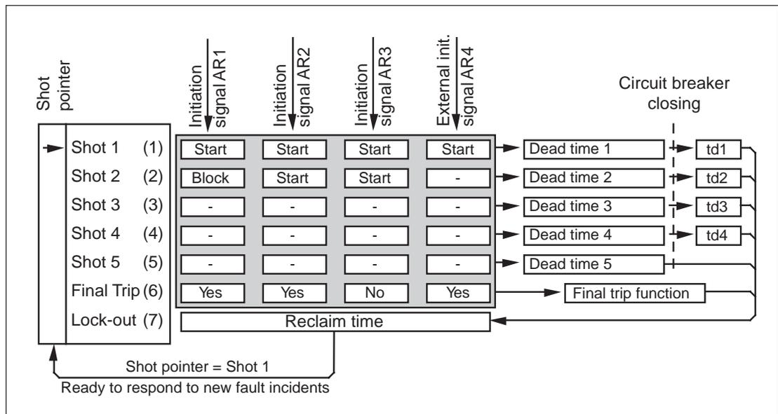
Fig. 3. Functional diagram for the auto-reclose relay module SPCT 5D54
