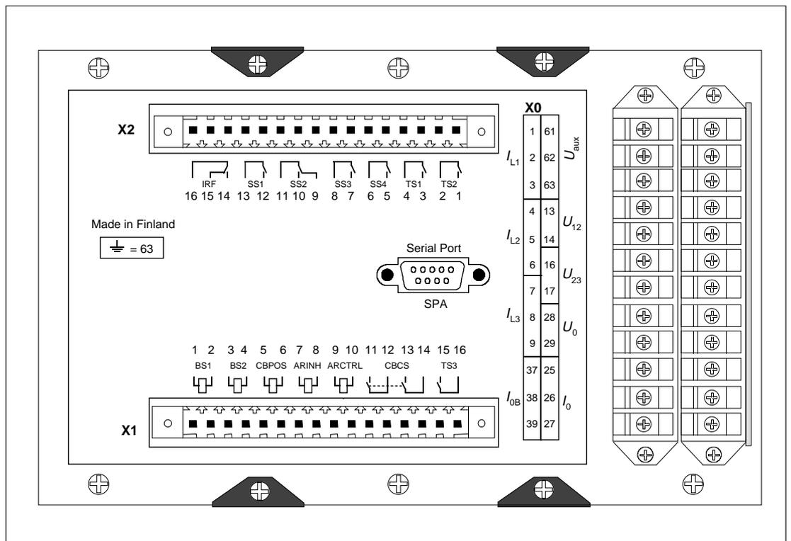
Fig. 2. Terminals of feeder protection relay SPAA 348 C.
