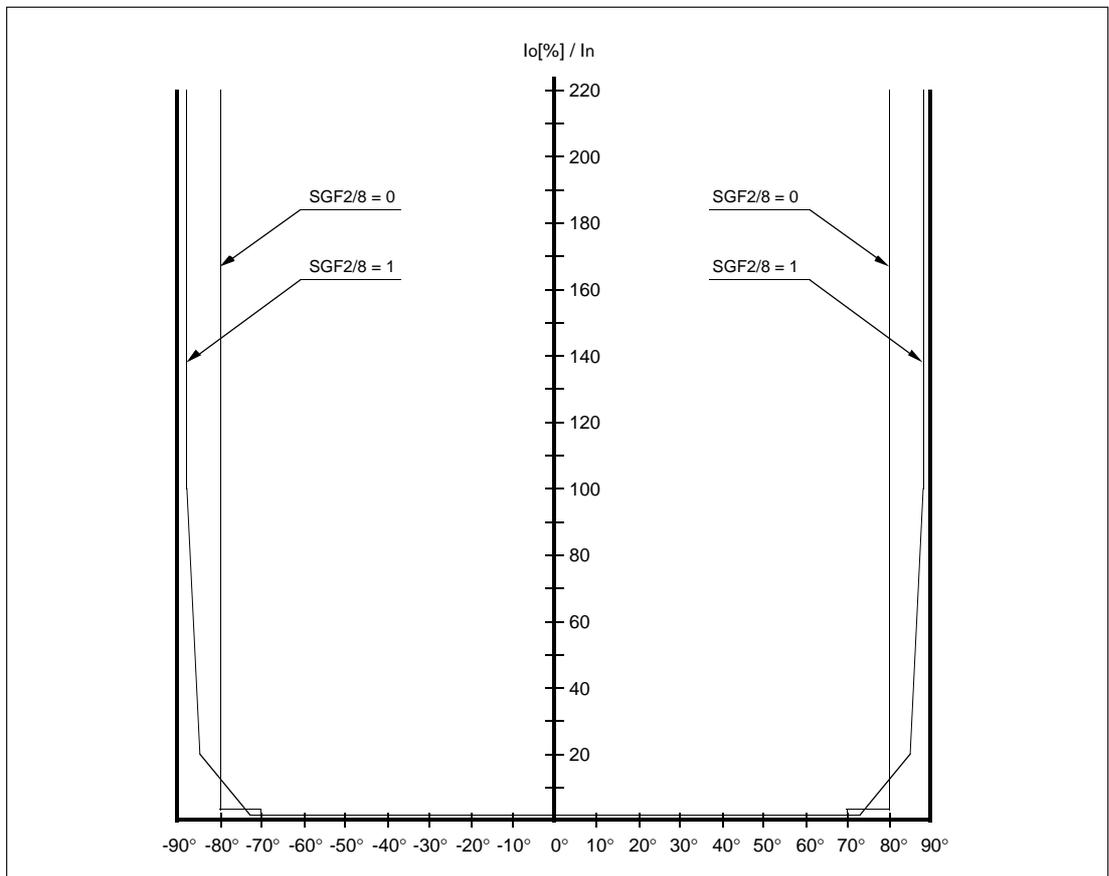
Fig. 1e. Operation characteristic of the directional earth-fault protection unit of the earth-fault relay module SPCS 2D26 illustrated in an  $I_0$ - $\varphi$  diagram, when the basic angle  $\varphi_b = 0^\circ$ .
