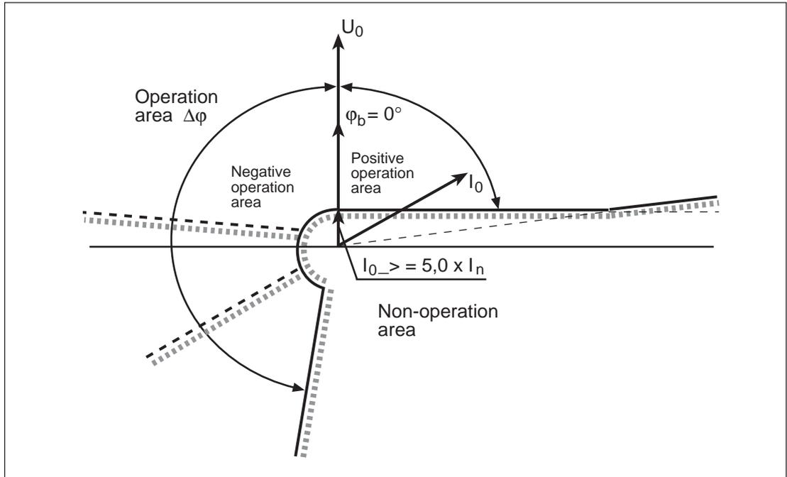
Fig.2. Example of two operation areas:  $\Delta\varphi$ ,  $-120^\circ \dots 0^\circ \dots +80^\circ$  &  $I_0 \cos \varphi$  and  $-170^\circ \dots 0^\circ \dots +80^\circ$  &  $I_0 \cos \varphi$ , when the basic angle  $\varphi_b = 0^\circ$ .
