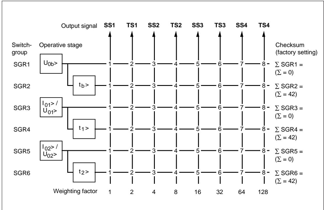
Fig. 7. Output relay matrix for earth-fault relay module SPCS 2D26
