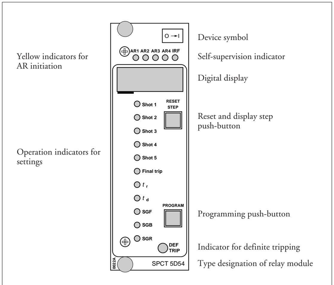
Fig.5. Front panel of auto-reclose module SPCT 5D54
