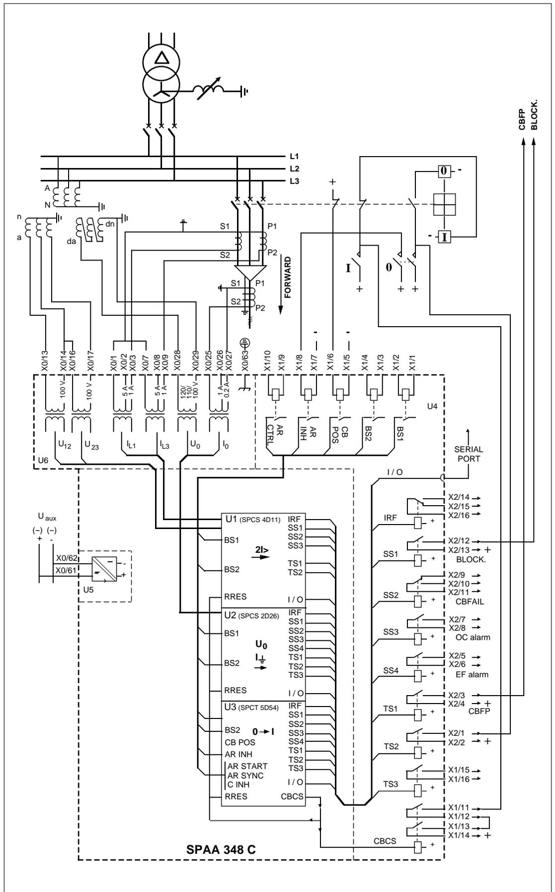
Fig. 6. Feeder protection relay SPAA 348 C used for protecting a feeder in a resonant earthed network.
