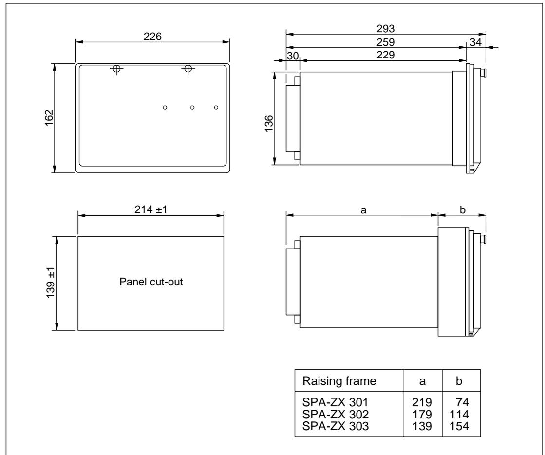
Fig. 16. Dimension and mounting drawings for feeder protection relay SPA 348 C.
