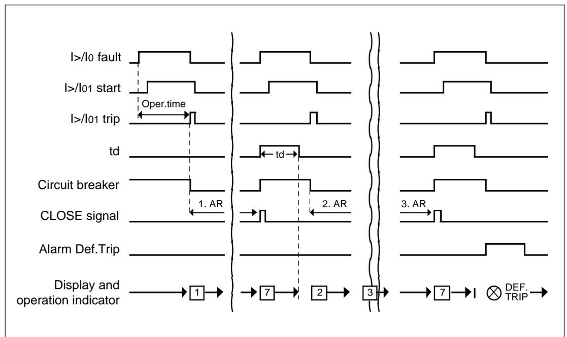
Fig. 8. Auto-reclose sequence when initiated by the start signal.
