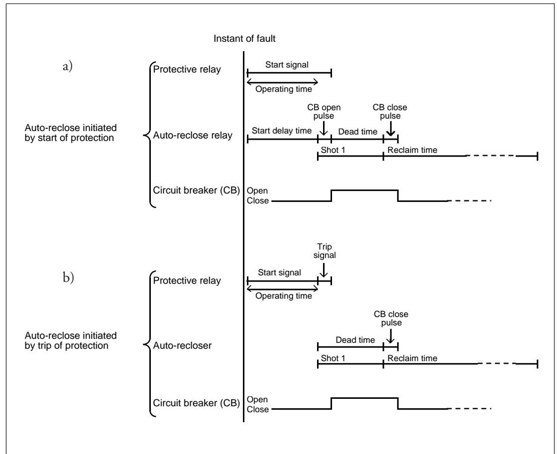
Fig. 1. Signal scheme illustrating the auto-reclose operation
