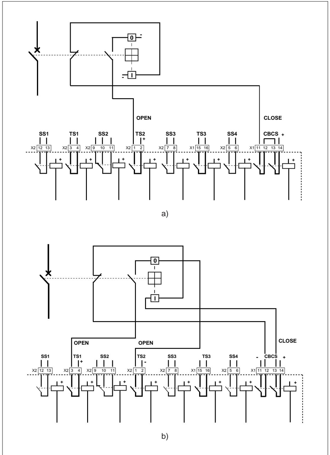
Fig. 3. Principle of one-pole (a) and double-pole (b) operation.
