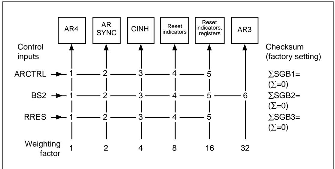
Fig. 6. Control signal matrix for auto-reclose module SPCT 5D54
