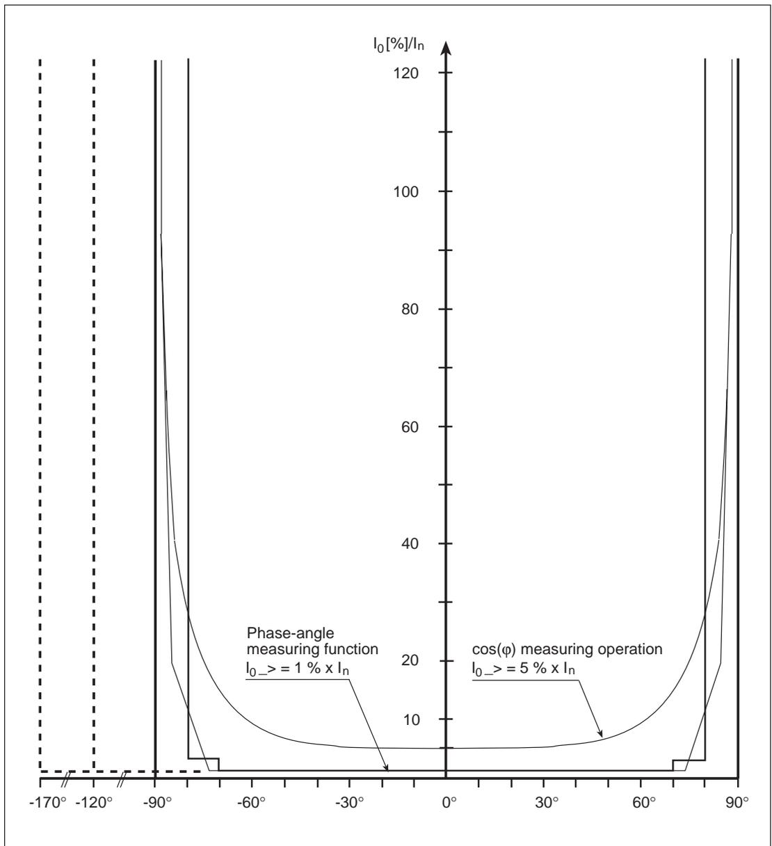
Fig.4 Overview of operation areas of the directional earth-fault stages, when the basic angle  $\varphi_b = 0^\circ$  and the start current  $I_{0\_>} = 1.0\% \times I_n$  at phase-angle measuring function and  $5.0\% \times I_n$  at  $I_0 \cos \varphi$  measuring function.
