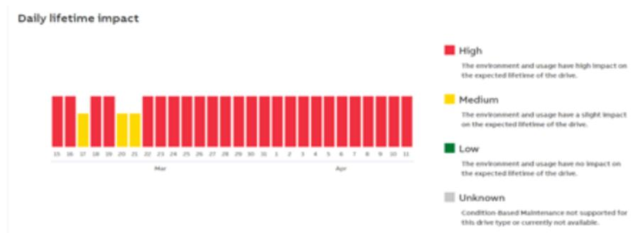
Figure 2: Analysis of the daily lifetime impact of the load on the drive operation.
