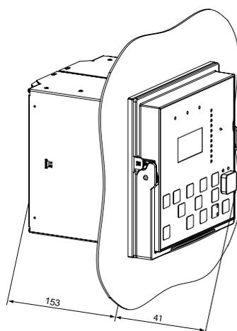
Fig. 7 Flush mounting
