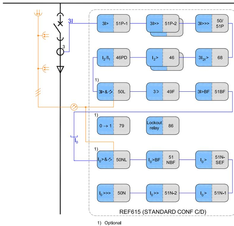
Fig. 2 Protection function overview of standard configuration C and D
