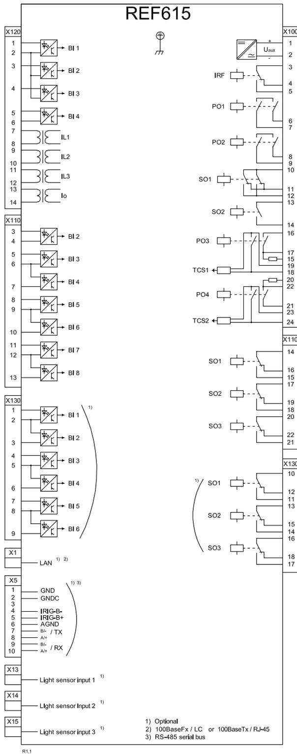
Fig. 12: Terminal diagram of standard configuration D
