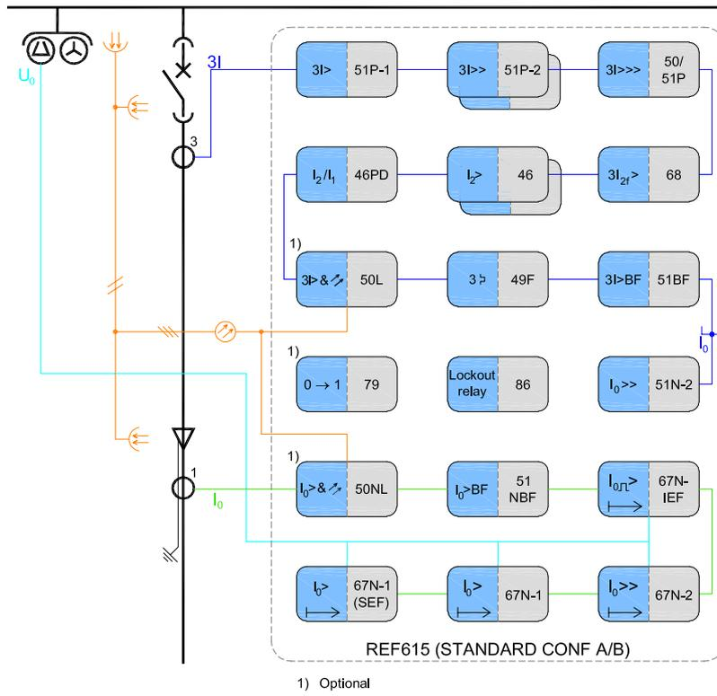
Fig. 1 Protection function overview of standard configuration A and B
