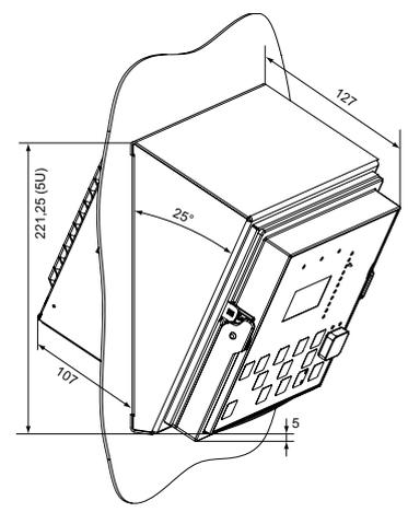
Fig. 9 Semi-flush with a 25° tilt
