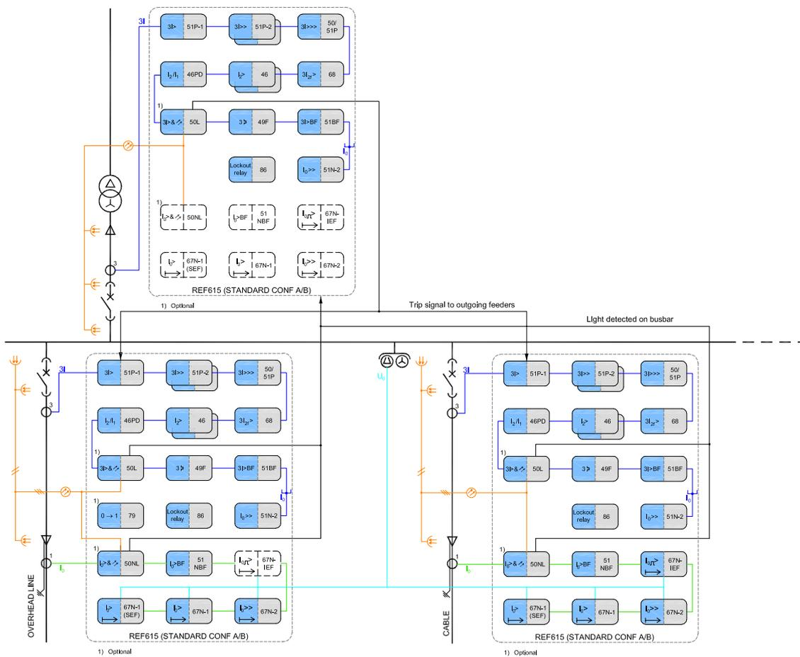
*Fig. 3 Substation O/C and E/F protection using the standard configuration A or B with relevant options. In the incoming feeder bay, the protection functions not used are uncoloured and indicated with a dashed block outline. The relays are equipped with optional arc protection functions, enabling fast and selective arc protection throughout the switchgear.*
