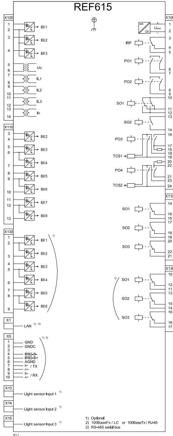
Fig. 11: Terminal diagram of standard configuration B
