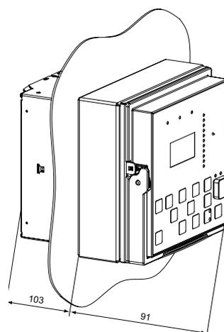
Fig. 8 Semi-flush mounting
