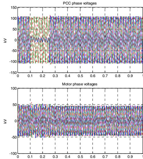
Figure 7 Single phase fault outside Kollsnes
