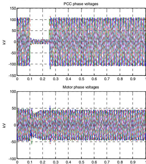
Figure 6 Three phase fault outside Kollsnes
