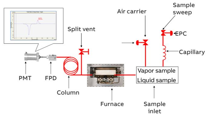
Figure 2 Operating diagram of the analysis system (sample injection, oxidation, separation, measurement)
