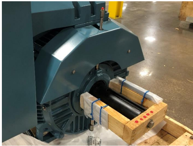
Figure 15 Option 1 – wooden rotor locking device
