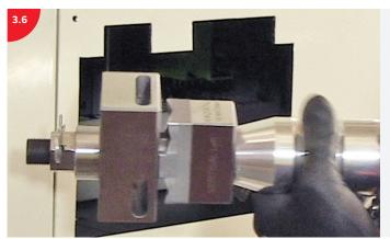
Note the cutting order. Cut the parts next to the edges first and the middle part last.
