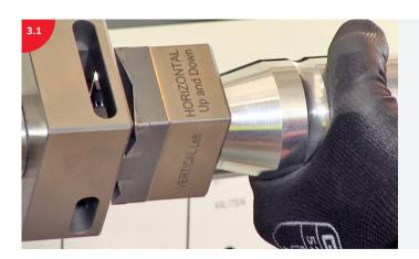
Ensure that the cutting head is set in the correct position. The text **HORIZONTAL Up and Down** must point in the direction you are cutting.
