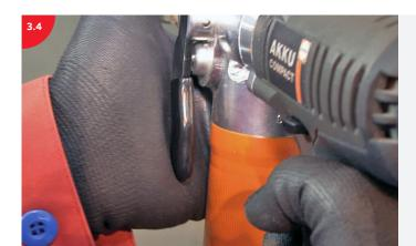
Push the vent lever to release the punch after each cutting cycle.
