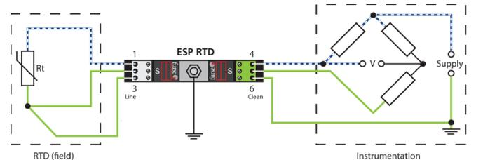
This could be accomplished using two ESP 06D or ESP SL06 SPDs where only 1 channel of the second SPD is utilised. However, this would be bulky and not cost effective due to the unused channel.
