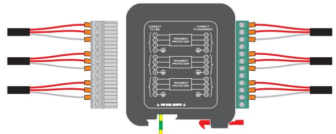
An ESP RTDQ unit is designed to protect up to three 3 wire systems with an earthed bridge.
