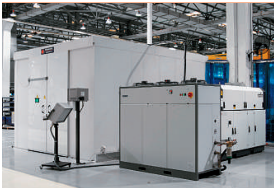
3 The laser can cause blindness – the cell is totally enclosed.
