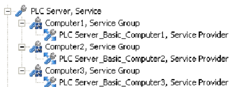
Figure 39. Service Structure Example
