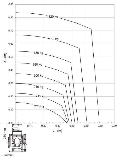
1.5.3 Maximum load and moment of inertia for full and limited axis 5 (center line down) movement
