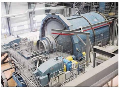
ABB AMI630 four-pole squirrel-cage asynchronous motor was illustrated. Part two focuses on field measurements taken from the drive system of an installed and commissioned  $2 \times 5$  MW dual-pinion ring-geared pebble mill  $\rightarrow$  1.
