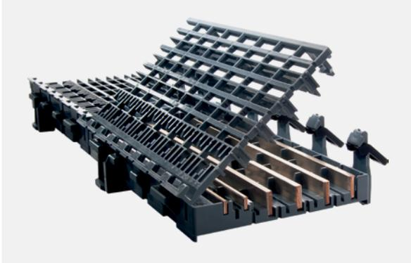
125A rated current side feeding socket system with integrated busbars for L1, L2, L3, N and 2 busbars for signalization. Additional socket with N and PE busbars.
