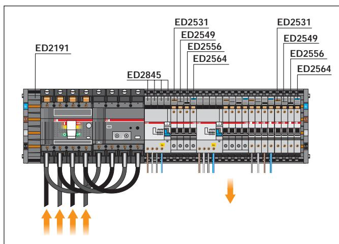
Busbar power supply from the top by means of 4P feeder module placed centrally
