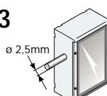
Protection against the penetration of solid bodies with a diameter or thickness of over 2.5 mm
