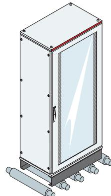
In the case of structures W=800mm (with internal or external cable container) containing busbar systems, check the centre of gravity before handling.
