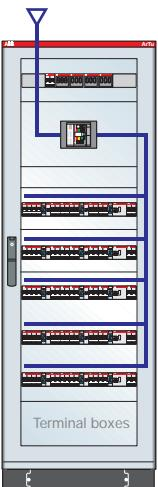
**ArTu K Series dim. 1800x600x350 (2031x748x225) mm (external hwxwd) IP65 with plate for Isomax S5 and modular panels, complete with 800A busbars vertically on back of structure - lcw max 35kA**
