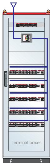
**ArTu M Series dim. 2000x600x250 (2196x724x250) mm (external hxwxd) IP65 with plate for Tmax T5 and modular panels, complete with 400A vertical busbars on back of structure - max. Icw 35kA**
