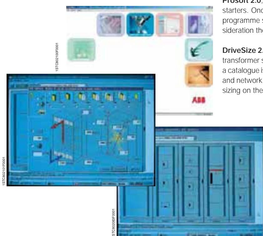
**DOCWin 3.0**, for sizing electrical networks powered with low or medium voltage, offers: design and definition of the network, network calculations, conductor sizing, selection and coordination of switching and protection devices, representation of the curves, checks, printout of diagrams, diagrams and reports;
