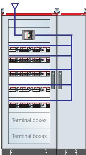
ArTu L Series dim.1600x900x195 (1750x1080x240) mm (external hwxwd) IP43 with cable container, plate for Tmax T3, modular panels Icw 25kA complete with busbar holder, 400A busbars, connections to the circuit-breaker, Unifix H and L
