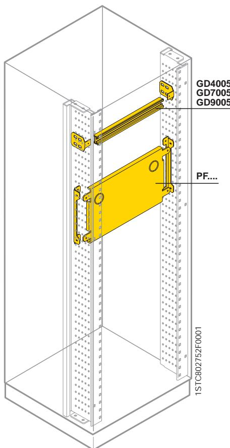
DIN rail kits for System Pro-M modular, Tmax T1-T2-T3, moulded-case circuit-breakers
