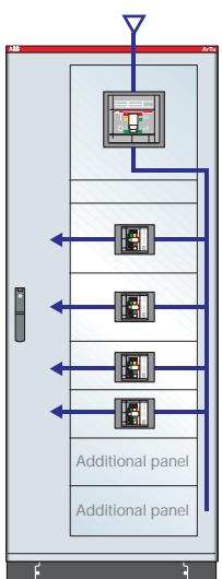
**ArTu K Series dim. 2000x800x500 (2231x948x637)mm (external hxwxd) IP65 with kit for Tmax T6, T3, T2, complete with 1600A busbars vertically on side on side of internal cable riser - Icw max 65kA**
