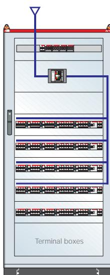
**ArTu M Series dim. 2000x800x250 (2196x924x250)mm (external hxwxd) IP65 with plate for Tmax T5 and modular panels, complete with 800A vertical busbars on back of structure- max. Icw 35kA**
