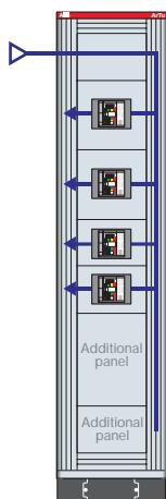
**ArTu K Series Form 3/4 segregation dim.1800x390x700 (2031x538x837) mm (external hwxw) IP31 with plate for Tmax T5, T3, T2 and modular panels, complete with 1600A busbars vertically on side of structure - lcw max 50kA**
