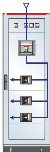
**ArTu K Series dim. 1800x600x500 (2031x748x637) mm (external hwxwd) IP41 with plate for Isamax S7, Tmax T5, T2 and modular panels, complete with 1250A busbars vertically on back of structure - lcw max 50kA**
