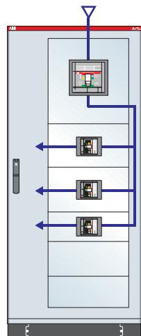
**ArTu K Series dim. 1800x800x500 (2031x948x637) mm (external hxwxd) IP41 with plate Tmax T7, T5, T2 and modular panels, complete with 1250A busbars vertically on side of internal cable riser - Icw max 35kA**
