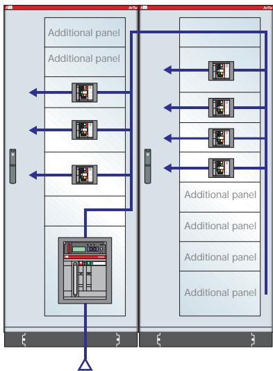
**ArTu K Series 2 x dim.2000x1600x700 (2231x1924x837) mm (external hxwxd) IP65 complete with 3200A horizontal and 1250A vertical busbars - Icw max 75kA**
