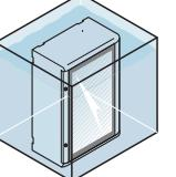
Protection against the penetration of water during continual immersion
