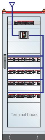
**ArTu M Series dim. 1800x600x250 (1996x724x250) mm (external hwxwd) IP65 with plate for Tmax T3 and modular panels, complete with 400A vertical busbars on back of structure - max. Icw 35kA**
