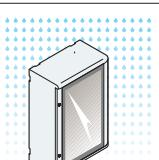
Protection against the penetration of drops of water falling vertically
