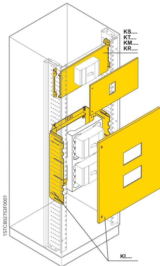
Kits for installing Tmax circuit-breakers
