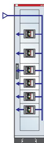
**ArTu K Series dim. 1800x390x500 (2031x538x637) mm (external hwxwd) IP41 with plate for Tmax T5, T3, T2 and modular panels, complete with 1250A busbars vertically on side of structure - lcw max 50kA**
