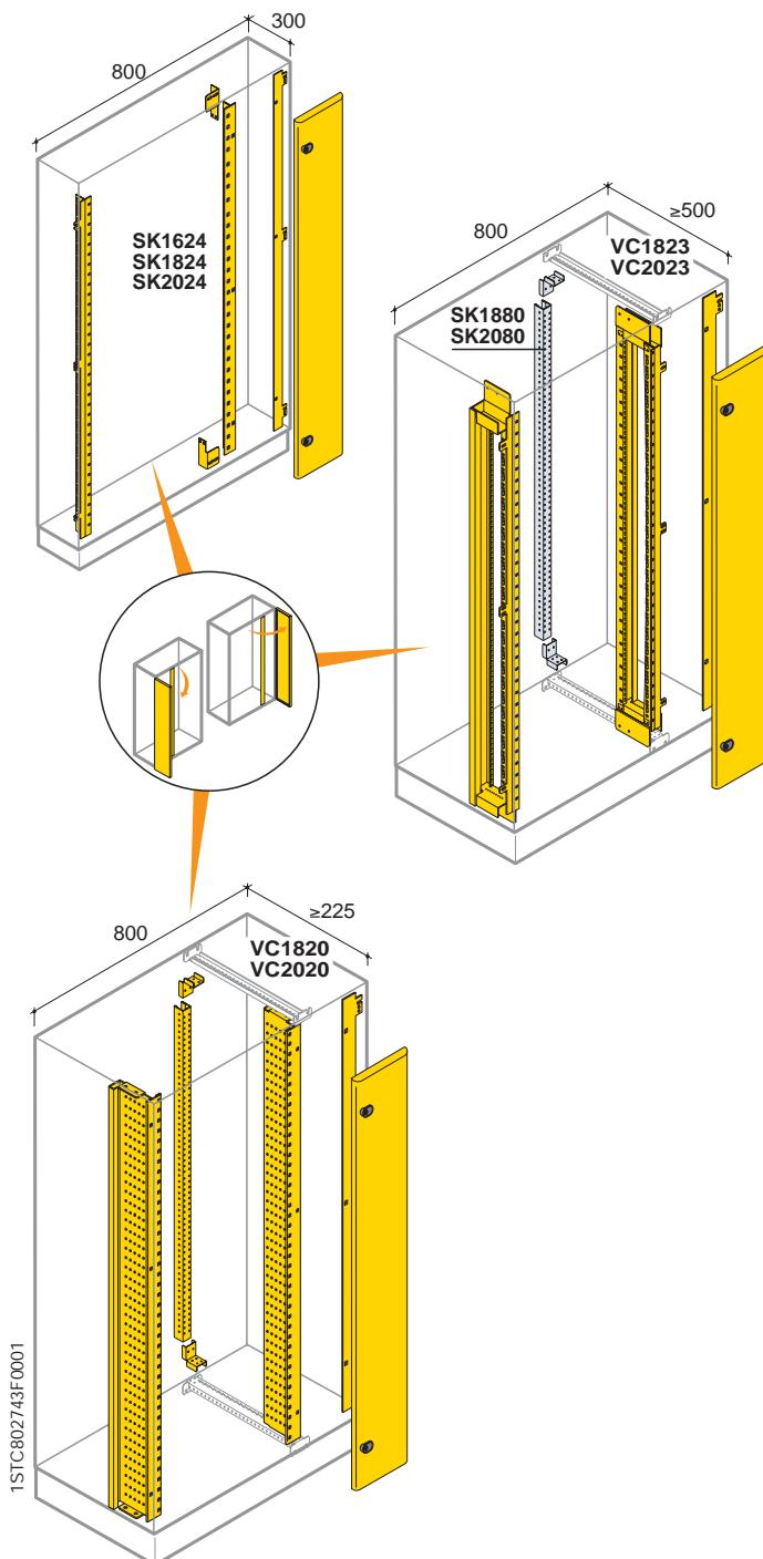
Internal cable container for switchgear without segregation (open frame)
