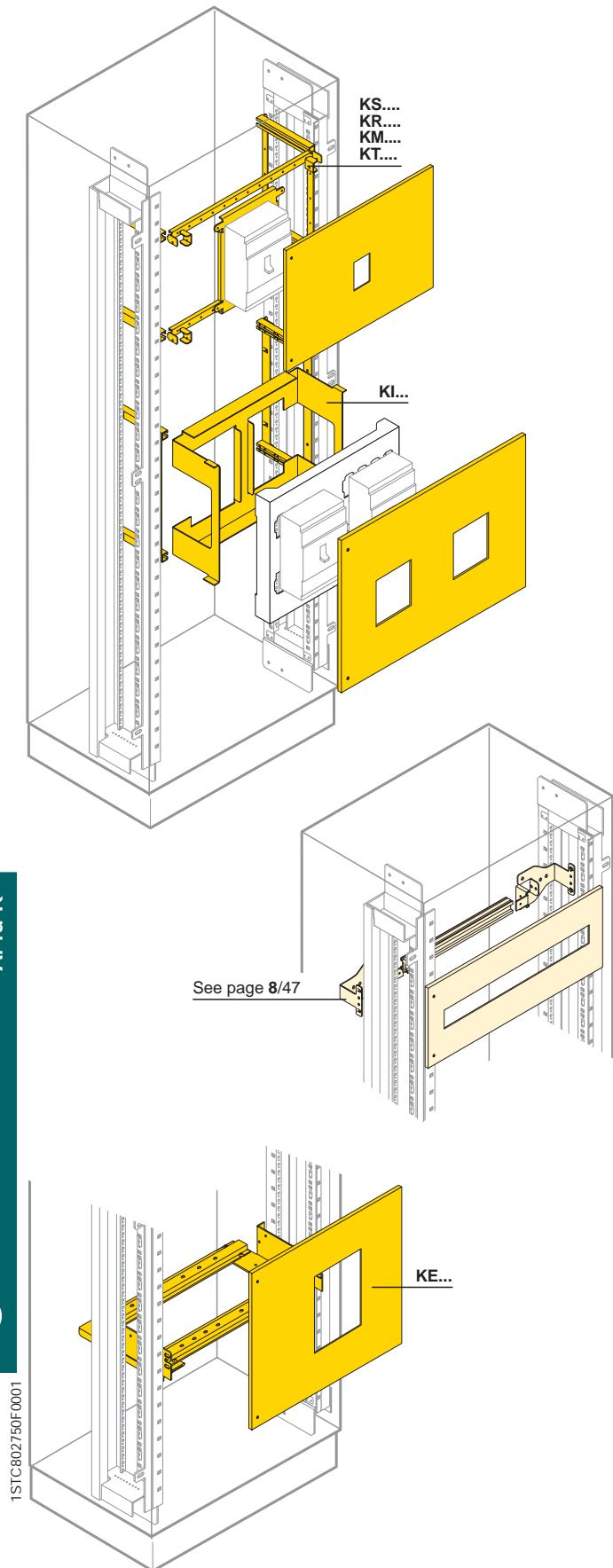
Kits for installing Tmax circuit-breakers
