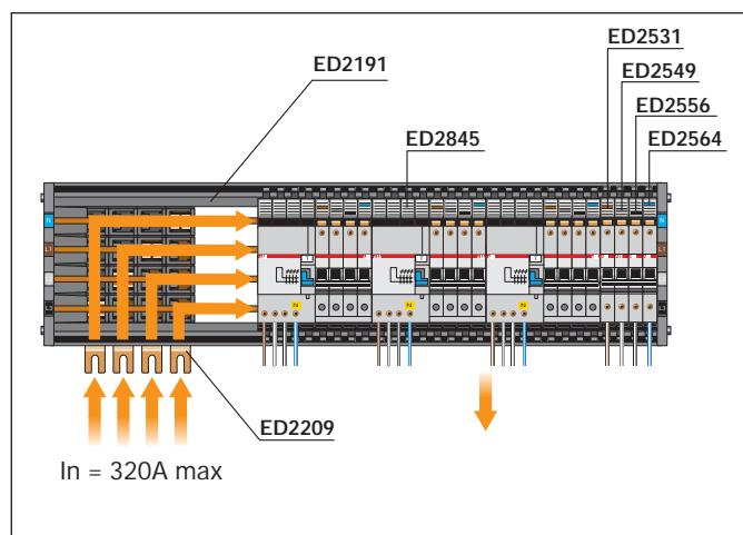
Busbar power supply from the bottom by means of main row circuit-breaker
