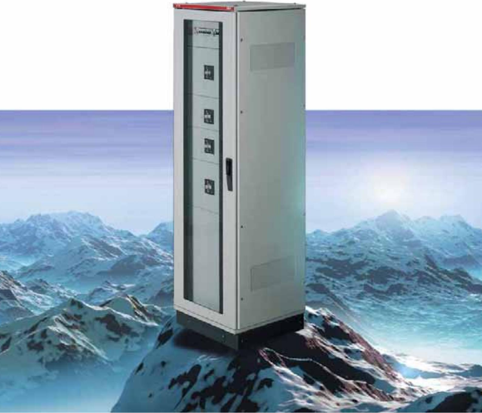
cuit-breakers, Tmax moulded-case circuit-breakers and Emax air circuit-breakers) with an excellent and certified level of integration. The switchgear is available in three functional widths (390, 600 and 800mm) and in two functional heights (1800 and 2000mm), which allow installation of 9 and 10 modules 200mm in height respectively.
