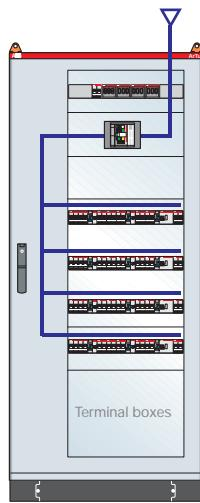
**ArTu M Series dim. 1800x800x250 (1996x924x250) mm (external hwxwd) IP65 with plate for Tmax T3 and modular panels, complete with 800A vertical busbars on back of internal cable container - max. Icw 35kA**
