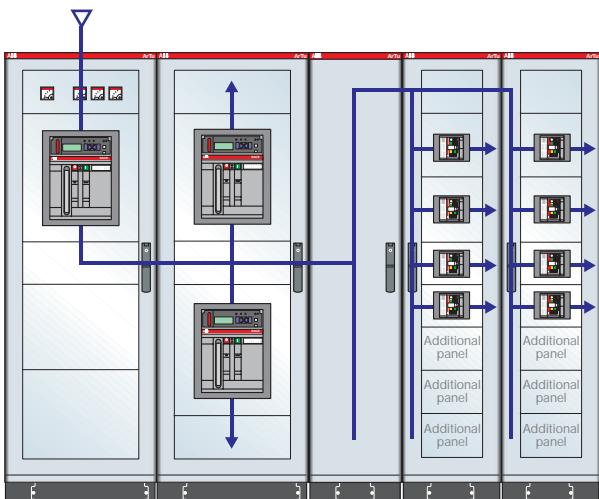
**ArTu K Series dim. 1800x2280x700 (2031x2904x837) mm (external hwxwxd) IP65 with Emax E1, T5 and T3, 1600A omnibus busbars and vertical 1250A branches - Icw 50kA**
