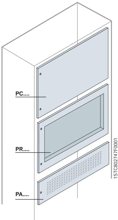
Blind, recessed and ventilated panels for general apparatus
