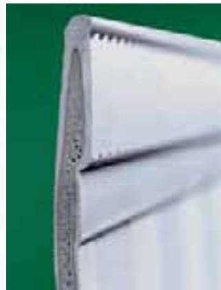
Gemini switchboards are made with co-injection, which ABB SACE is the first manufacturer in the electric field to use as a molding technique. This process obtains a "sandwich" of two materials with a compact external covering and an expanded core, guaranteeing the highest level of mechanical protection against impacts (IK10) without the need to add hardening substances.
