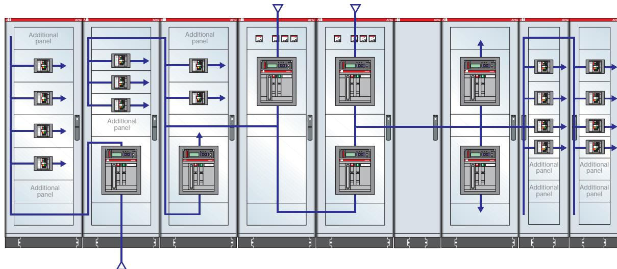
**ArTu K Series dim. 1800x4680x900 (2031x5804x1037) mm. (external hwxwd) IP65 with Emax E3, T5 and T33200A omnibus busbars and vertical 1600A branches - Icw 50kA**
