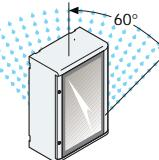
Protection against the penetration of drops of water falling at an angle of up to 60° from vertical
