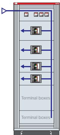
**ArTu K Series Form 3/4 segregation dim.1800x600x700 (2031x748x837) mm (external hwxwxd) IP31 with plate for Tmax T5, T3, T2, complete with 1600A busbars vertically on side of structure - Icw max 50kA**
