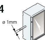
Protection against the penetration of solid bodies with a diameter or thickness of over 1.0 mm
