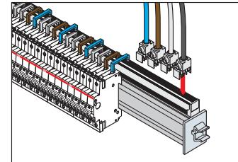
Power supply of the busbar with 100A feeder module without cable. Terminal capacity 35mm<sup>2</sup>.
