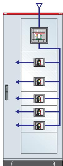
**ArTu K Series dim. 2000x800x500 (2231x948x637)mm (external hxwxd) P41 with kit for Tmax T6, T5, T3, complete with 1600A busbars vertically on side on side of internal cable riser - Icw max 65kA**
