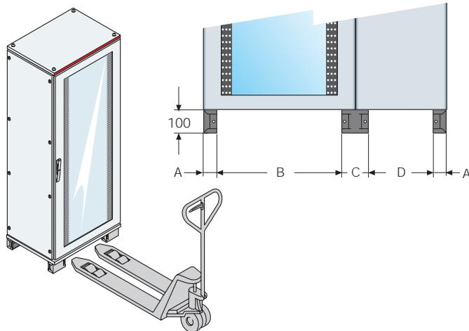
For greater safety during transport using a fork-lift truck, it is advisable to anchor the switchgear to the truck:
