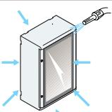
Protection against the penetration of water sprayed by a hose from all directions
