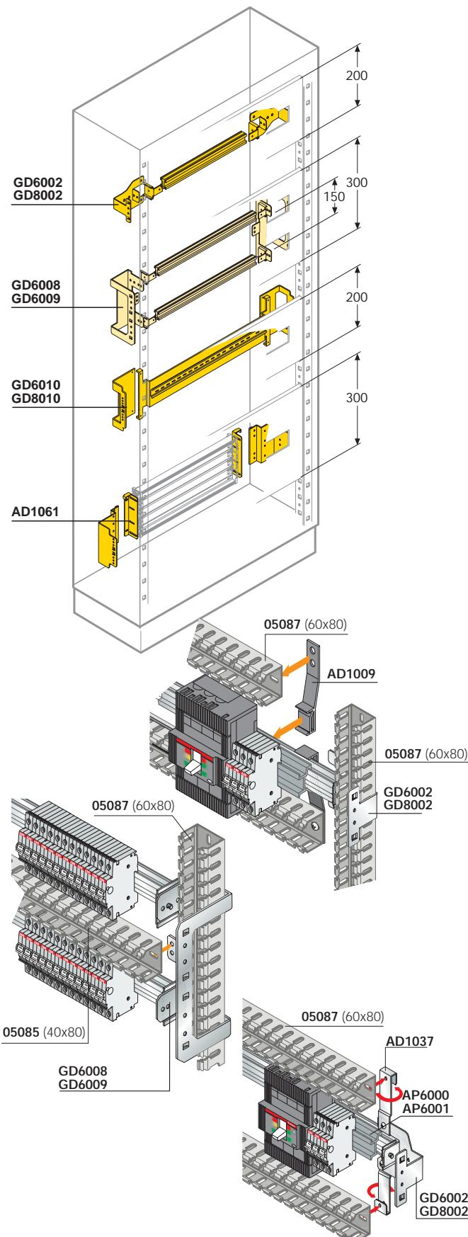
DIN rail kits for System Pro-M modular apparatus, Tmax T1-T2-T3, moulded-case circuit-breakers and supports for Unifix H
