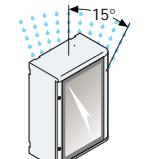
Protection against the penetration of drops of water falling at an angle of up to 15° from vertical
