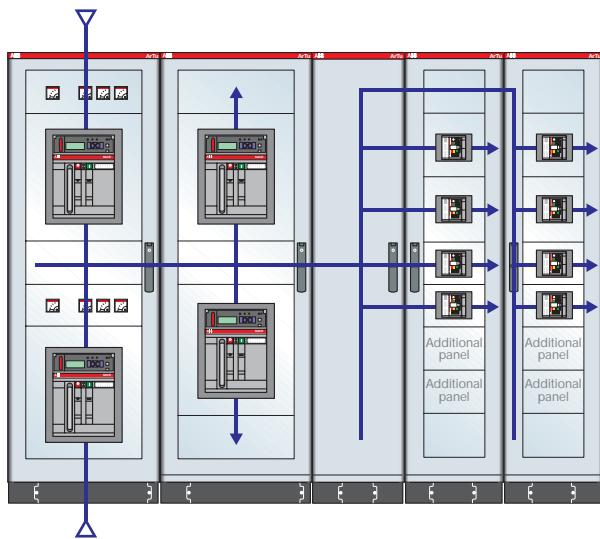
**ArTu K Series dim. 1800x2280x700 (2031x2900x837) mm (external hwxwd) IP65 with Emax E2, T5 and T3, 3200A omnibus busbars and vertical 1600A branches - Icw 65kA**
