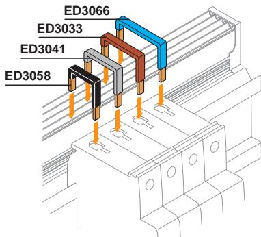
**Connections for various apparatus**
