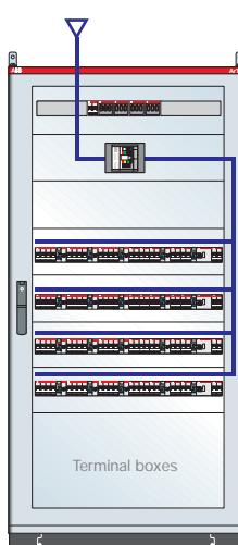
**ArTu K Series dim. 1800x800x150 (2031x948x287) mm (external hxwxd) IP65 with plate for Tmax T3 and modular panels, complete with 800A busbars vertically on back of internal cable cont. - Icw max 35kA**
