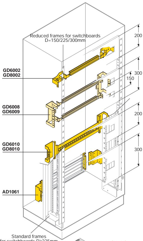
DIN rail kits for System Pro-M modular, Tmax T1-T2-T3, moulded-case circuit-breakers for Unifix H
