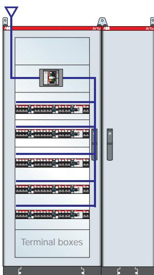
ArTu L Series dim. 1800x900x195 (1950x1080x240) mm (external hxwxd) IP43 complete with cable container l=300mm, plate for Tmax T3 and modular panels
