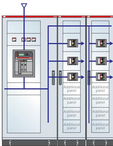
**ArTu K Series dim. 1800x1580x700 (2031x1984x837) mm (external hxwxd) IP65 with Emax E1, T5 and T3, 1600A omnibus busbars and vertical 800A branches - lcw 50kA**
