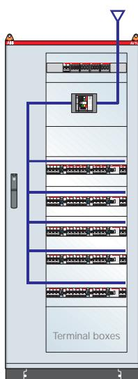
**ArTu M Series dim. 2000x800x250 (2196x924x250) mm (external hxwxd) IP65 with plate for Tmax T5 and modular panels, complete with 800A vertical busbars on back of internal cable container - max. Icw 35kA**
