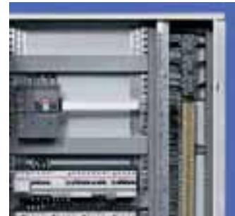
The 400 and 800A busbar system with shaped section, with prefabricated connections between circuit-breakers and busbars placed in the various situations can be used. It is always possible to use the traditional flat busbars for capacities up to 630A. The degree of protection goes from IP31, for the versions without door, up to IP43 for the versions with door.
