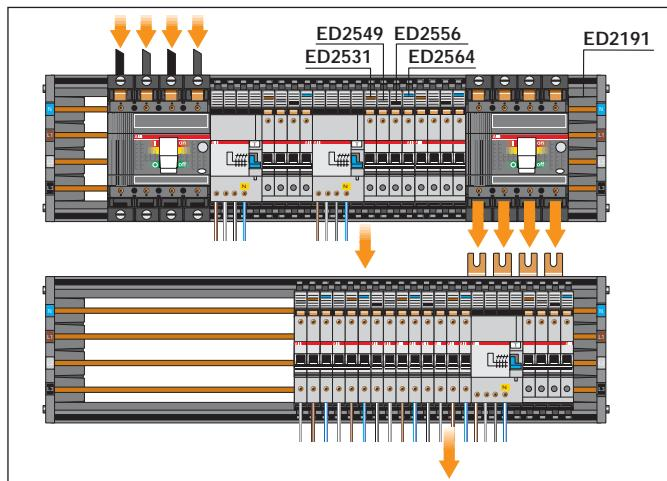
Busbar power supply from the bottom by means of 4P feeder module placed laterally
