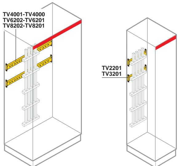
Fixing crosspieces for busbars with shaped section
