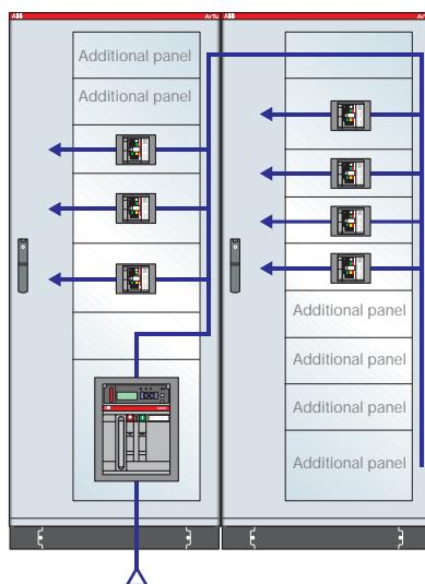
**ArTu K Series 2 x dim.2000x1600x700 (2231x1924x837) mm (external hxwxd) IP65 complete with 1600A horizontal and 1250A vertical busbars - Icw max 75kA**
