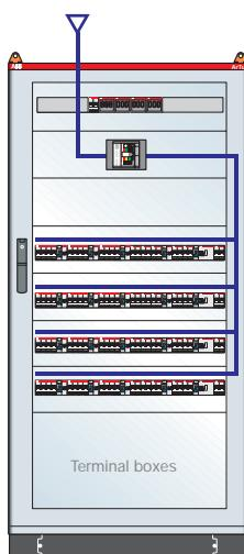
**ArTu M Series dim. 1800x800x250 (1996x924x250) mm (external hwxwd) IP65 with plate for Tmax T3 and modular panels, complete with 800A vertical busbars on back of structure - max. Icw 35kA**
