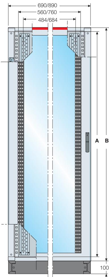
Front of structure with internal cable container
