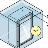
Protection against the penetration of water during temporary immersion
