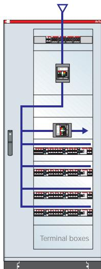
**ArTu K Series dim. 2000x800x300 (2231x948x437)mm (external hwxwd) IP65 with plate for Tmax T5, T2 and modular panels, complete with 400A busbars vertically on back of structure - lcw max 35kA**
