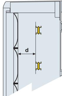
The distances of the DIN rail from the panel depend on the depth at which the DIN rail is regulated by using fixing devices.
