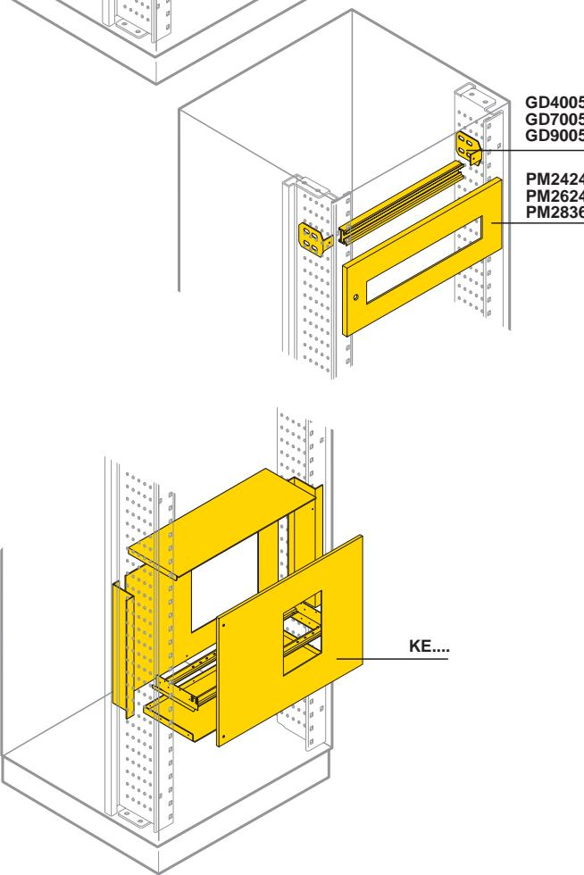
Kit for installation of Tmax circuit-breakers
