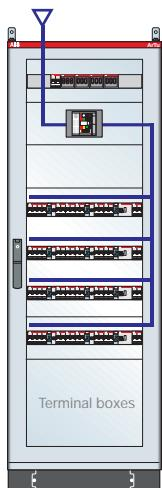
**ArTu K Series dim. 1800x600x150 (2031x748x287) mm (external hxwxd) IP65 with plate for Tmax T5 and modular panels, complete with 400A busbars vertically on back of structure - Icw max 35kA**
