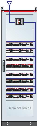
**ArTu K Series dim. 2000x600x150 (2131x748x287) mm (external hwxwd) IP65 with plate for Tmax T5-630A and modular panels, complete with 400A busbars vertically on back of structure - lcw max 35kA**
