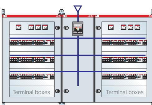
**ArTu L Series dim.1000x1500x165 (1050x1770x204) mm (external hwxwd) IP43 with cable container, plate for Tmax T3, modular panels Icw 16kA complete with busbar holder, 250A busbars and Unifix L**
