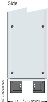
Handling ArTu K structures by means of rollers: only with **ZR...reinforced plinth**
