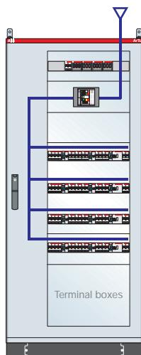
**ArTu K Series dim. 1800x800x150 (2031x948x287) mm (external hxwxd) IP65 with plate for Tmax T3 and modular panels, complete with 800A busbars vertically on back of internal cable cont. - Icw max 35kA**
