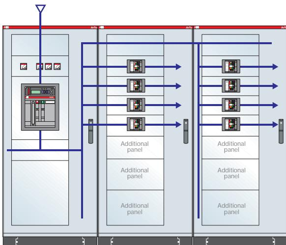
**ArTu K Series dim. 1800x2400x700 (2031x2784x837) mm (external hxwxd) IP65 with Emax E1, T4 and T1, 1600A omnibus busbars and vertical 1250A branches - Icw 50kA**
