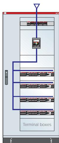
**ArTu K Series dim. 1800x800x225 (2031x948x362) mm (external hwxwd) IP65 with plate for Tmax T5 and modular panels, complete with 800A busbars vertically on side of int. cable container - lcw max 35kA**
