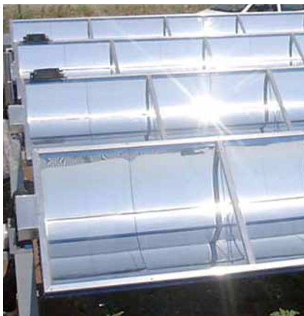
Figure B.5 – Parabolic trough concentrators
