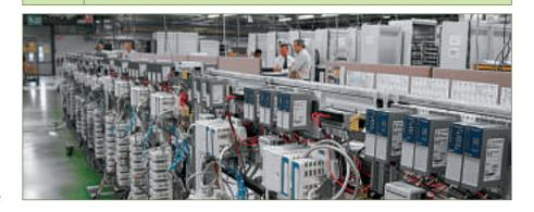
mounted in 'Ex-e' rated cabinets for zone one mounting. ABB is also supplying Introl control valves for all the platforms and variable speed drives are delivered for pump control.
