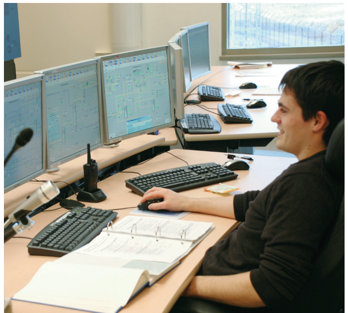
Illustration of the Ormen Lange gas field. Courtesy of Shell. | Operators are trained, and new processes and subsystems are designed, engineered, corrected and tested in the 800xA Simulator before they are integrated into the main control system.
