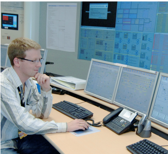
Illustration of the Ormen Lange gas field. Courtesy of Shell. | Operators are trained, and new processes and subsystems are designed, engineered, corrected and tested in the 800xA Simulator before they are integrated into the main control system.
