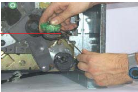
Disconnect the microswitch connection (4)
