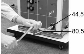
Figure 4.19 Manual charging of HD4 circuit-breaker springs.
