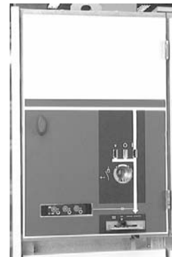
Figure 4.16 The door to the control and secondary apparatus compartment can be opened by turning the handle in a clockwise direction, and closed by turning in an anticlockwise direction.
