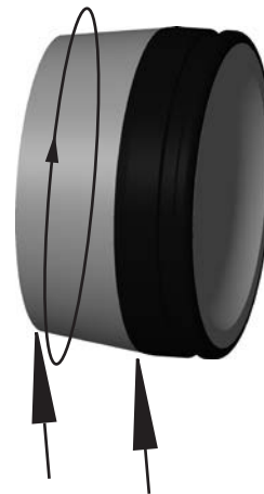
Fig. 2.1.3.3: Greasing the silicone insulating part of the voltage transformer in the area between the arrows
