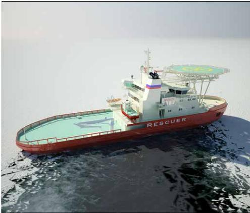
1:25 scale model, everything needs to be kept in line with the scale laws of the test. Even time is scaled; the captain has to make decisions at five times the normal speed.
