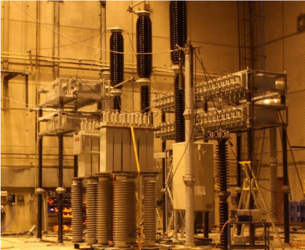
Figure 6. Test setup of MRTS with capacitor banks in front of and behind the three breaker poles connected in series.
