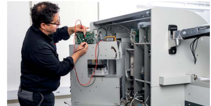
Figure 3: Automated paper testing systems that enable modules to be serviced while in operation ensure minimum impact to quality testing and continuous operation
