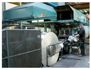
Operator Mr. Peter Lindström: "The MTG-gauge works very well. The only thing you have to think of is to do a new set up when you change strip thickness. The HMI screen is working well and is easy to operate".
