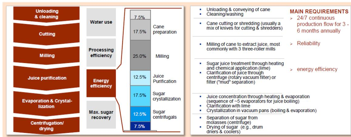
Figure 6: Energy consumption highlights in sugar production
