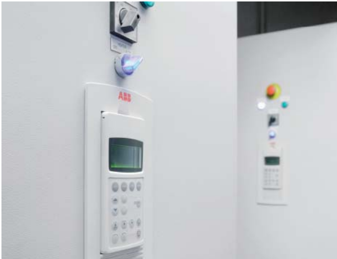
The winch control program inside ABB's ACS800 industrial drive was easily adapted to meet the needs on the m/s Viking Grace.
